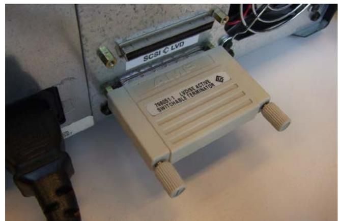
Figure 4: SCSI terminator attached to DLT-IV drive
