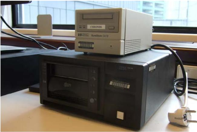
Figure 2: DLT-IV (bottom) and DDS-2 (top) tape drives
