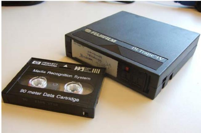
Figure 1: DDS-1 (left) and DLT-IV (right) tape
