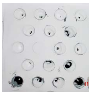
Fig.1 The ionizing stage with small electrode gap loaded with \text{Al}_2\text{O}_3 particles
