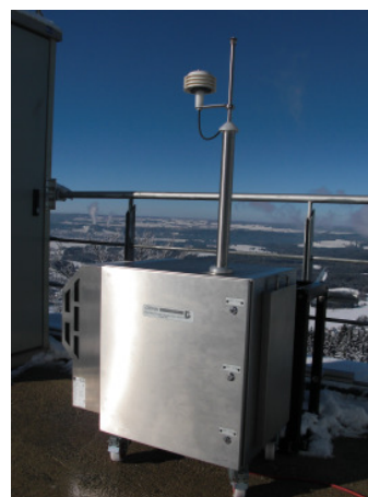
Figure 2. Installation of the WRAS system on the roof platform of the GAW station Hohenpeissenberg
