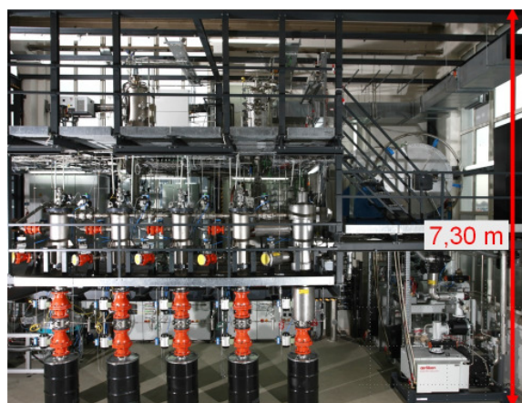
Figure 1: 3-level Nanoparticle synthesis plant: Filter system in front of the image on the ground level; reactors on the first and second level.
