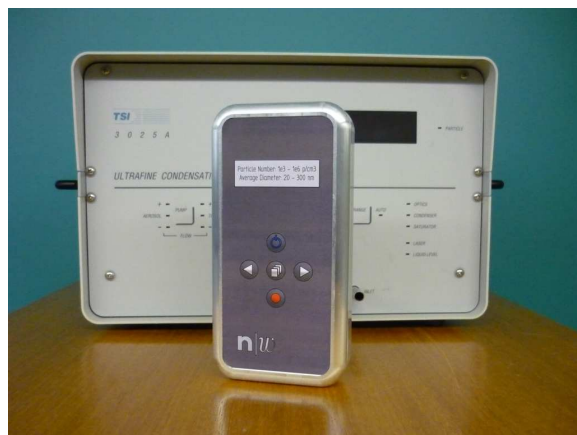
Figure 1: an image of the miniaturized diffusion size classifier (miniDiSC) compared to a CPC.
