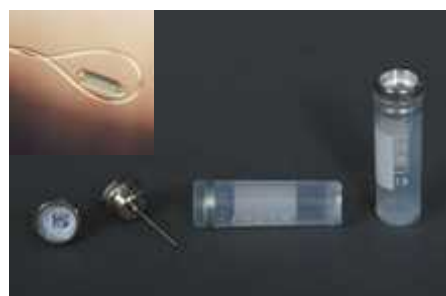
Fig. 2.8: Loop, crystal caps and vials as provided by Hampton Research.
