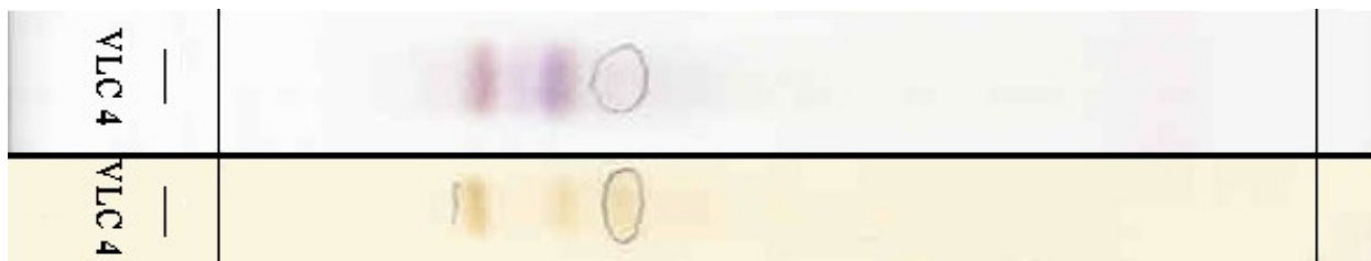
pict. 17; TLC spots of VLC 4. Plates sprayed with vanilla spray agent (upper plate), and \text{KMnO}_4 spray agent (lower plate).
