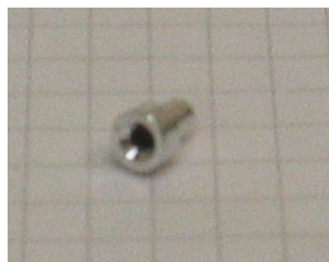
Figure 5.3.: Photograph of a target holder containing pulverized standard material.
