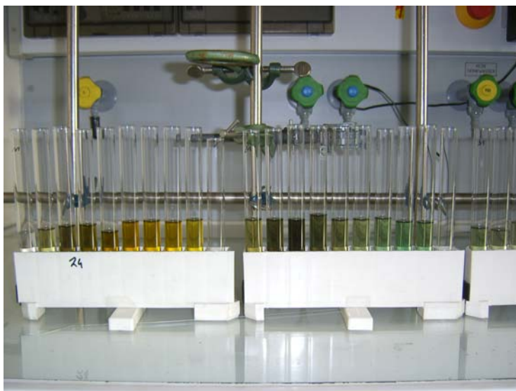
Figure 33: First obtained fractions of \text{CHCl}_3 extract by column chromatography
