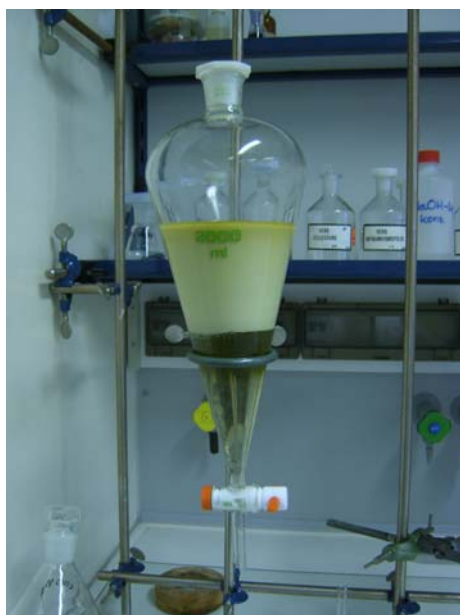
Figure 21: Partition of MeOH-H 2 O-layer with chloroform
