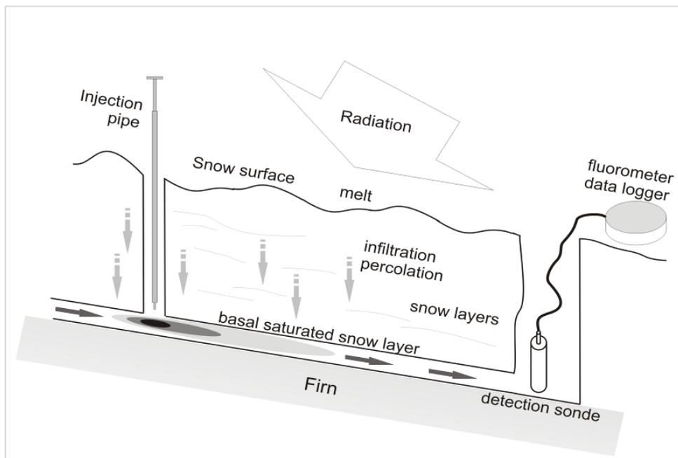
**Fig. 14:** Schematic figure; experimental configuration for dye tracer measurements on firn. Source: own illustration
