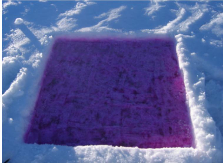
**Fig. 12:** Potassium Permanganate application on snow for permeability test; Source: own picture
