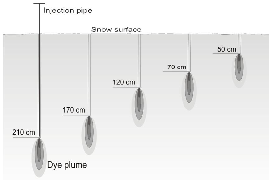
**Fig. 13:** Schematic view of dye injection into different snow depths with injection pipe. Source: own illustration
