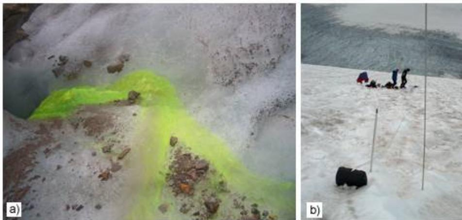
**Fig. 15:** a) Fluorescein release into glacier moulin at 'Oberer Boden' ; b) Dye tracer release into basal snow layer at experimental site 'Lieslstang'; injection pipe in the foreground, Source: own picture
