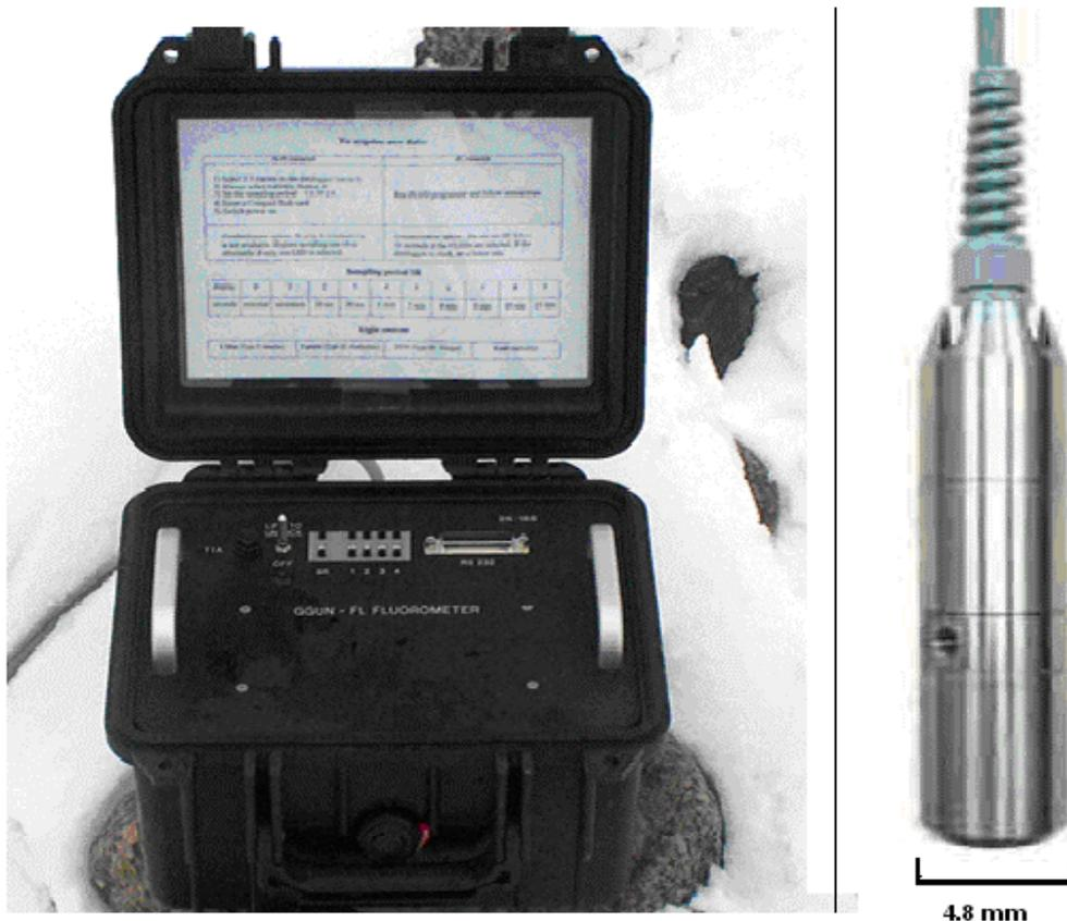
**Fig. 17:** Flow-through field fluorometer GGNU-FI and detection sonde. Source: own picture
