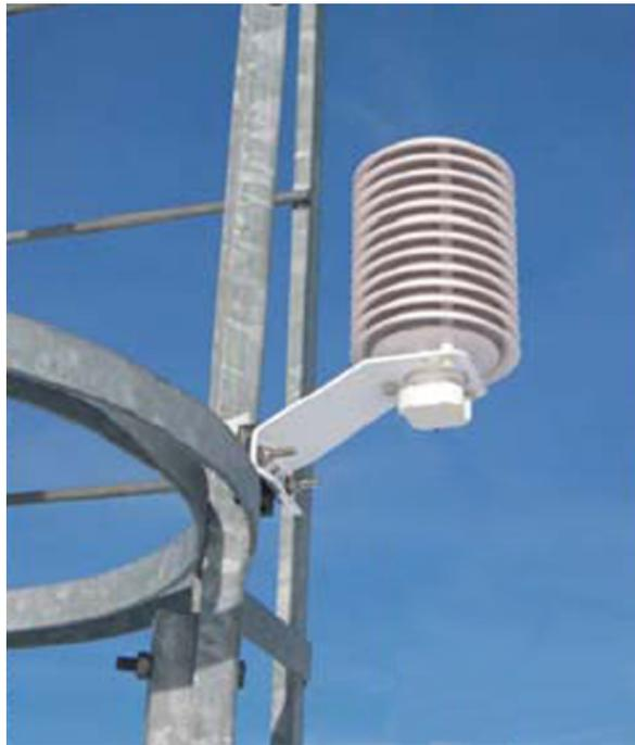
**Fig. 20:** Temperature sonde installed on the Observatory Hoher Sonnblick (3106m); Source: own picture
