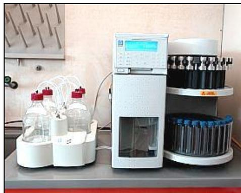
Abbildung 8: Probenzelle, Dionex ASE 200 - Accelerated Solvent Extractor
