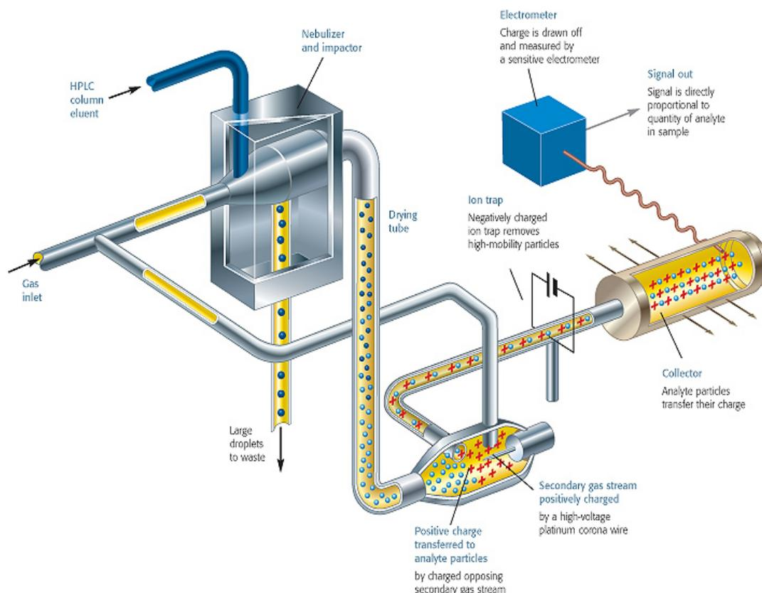
Figure 2: Illustration of the operation principle of the CAD.
