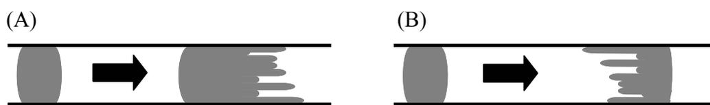
Figure 10: Demonstration of the band distortions due to the formation of viscous fingers. In (A) a plaque of lower viscosity solvent was injected. In (B) the introduced plaque exhibited a higher viscosity compared to the mobile phase.
