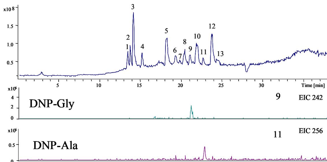
Figure 16: Chromatogram of fraction 2 of the tandem RP column derivatized with Sanger's reagent (2,4-dinitrofluorobenzene).
