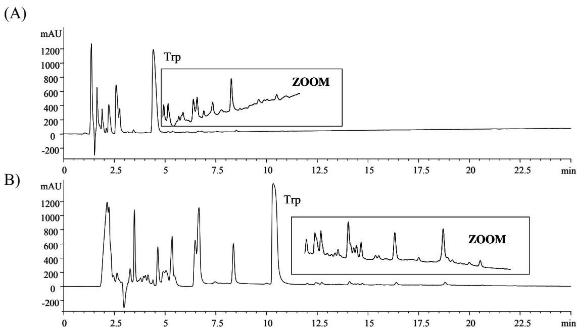
Figure 13: UV-chromatograms of a stressed infusion solution (stored at 60°C for 9 months) on (A) Chromolith RP18e and on (B) Gemini C18.
