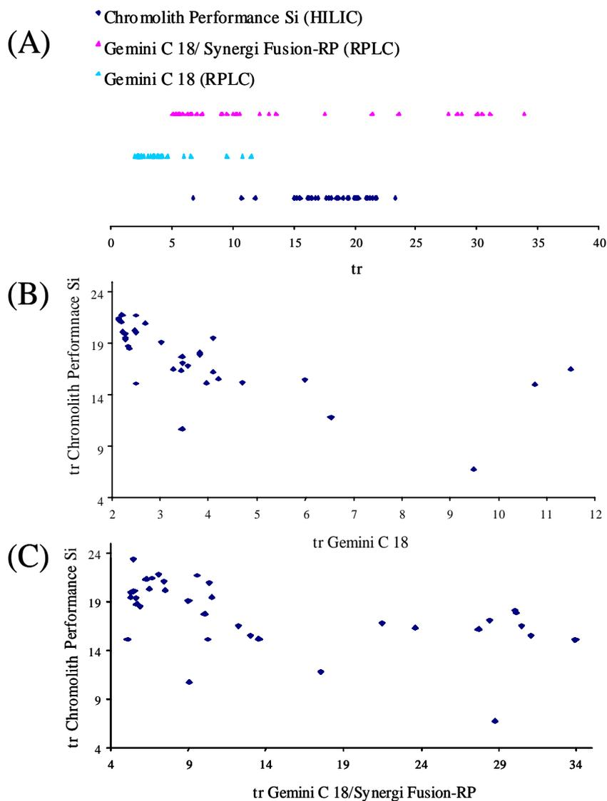
Figure 14: (A) 1-D plots of retention times on Gemini C18, tandem Gemini C18/Synergi Fusion-RP80 and Chromolith Performance Si. Complementarity plots of retention times on Chromolith Performance Si versus retention times on (B) Gemini C18 and on (C) tandem Gemini C18/Synergi Fusion-RP, respectively.
