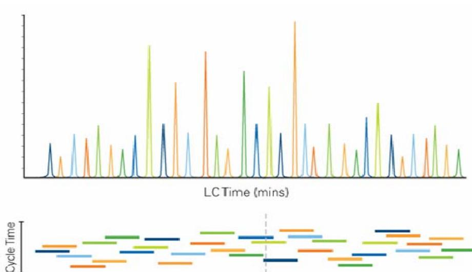
Figure 5: Illustration of the Scheduled MRM Algorithm.
