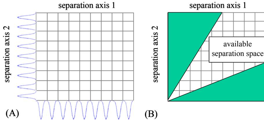
Figure 8: In scheme (A) on the left side the separation space of an idealized 2-D separation system is shown. Peaks are lined up one after the other at constant resolution.
