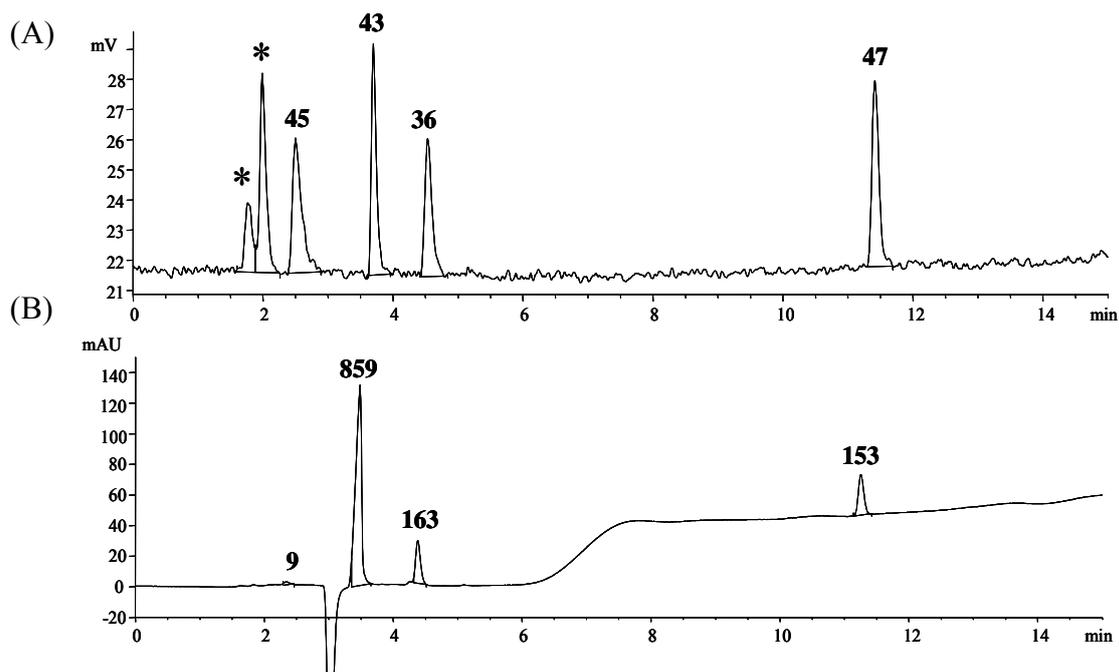
Figure 11: Chromatograms obtained with (A) CAD and (B) UV detector.
