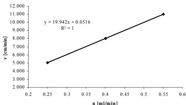
Figure 20: Plot of linear velocity versus flow rate on Luna Amino (150 x 3 mm; 5  $\mu$ m) using acetone as void time marker.
