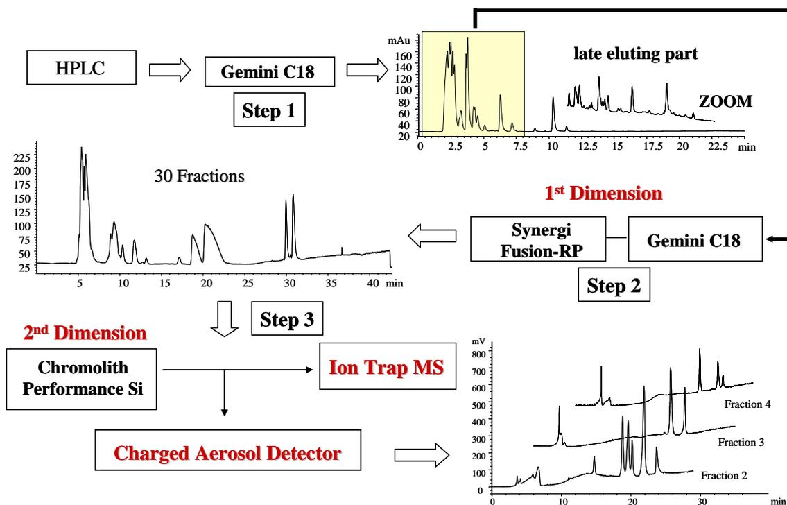
Figure 15: Schematic illustration of the work flow of the developed multidimensional analysis assay.
