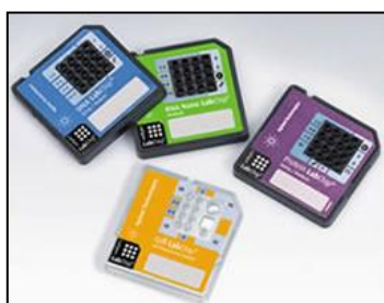
Fig. 10: Chips for Agilent 2100 Bioanalyzer – blue for DNA, green for RNA and violet for protein analysis. Yellow chips are employed for cell flow-cytometry. Image taken from http://www.bcm.edu/cms_web/110/biolabchips.jpg
