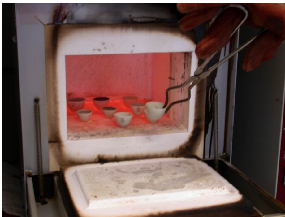
Figure 13: Determination of the ash content in the muffle furnace.
