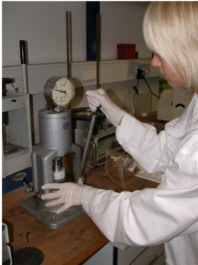
Figure 11: Pressing of the grinded material into pellets.
