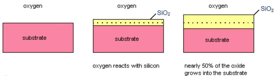
**Figure 9: growth behavior of oxide on silicon[54]**
