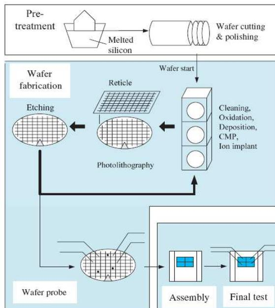
**Figure 6: generic survey of semiconductor manufacturing process[27]**
