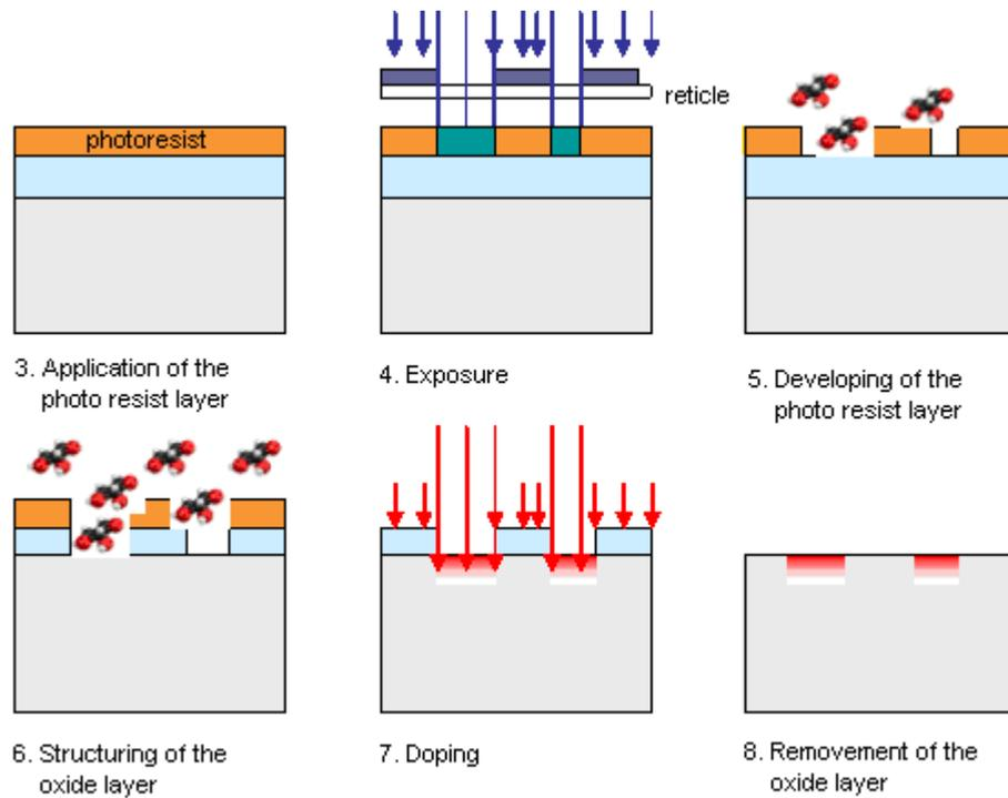
**Figure 7- 1: Fabrication of a single layer[35]**
