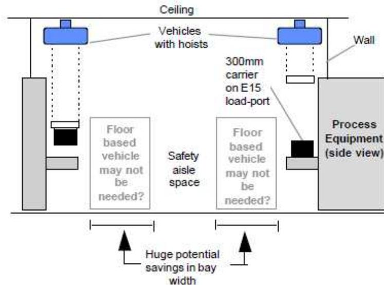
**Figure 24: Over hoist intra-bay material handling [55]**
