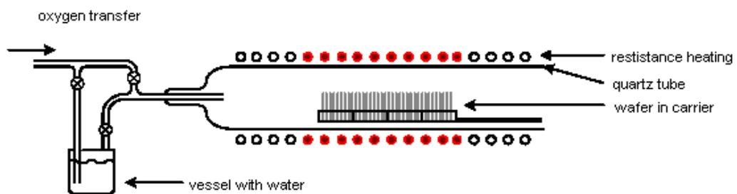
**Figure 8: Demonstration of a furnace for oxidation[54]**
