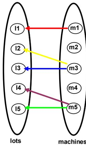
**Figure 17: Lot processing on machine without sequence**
