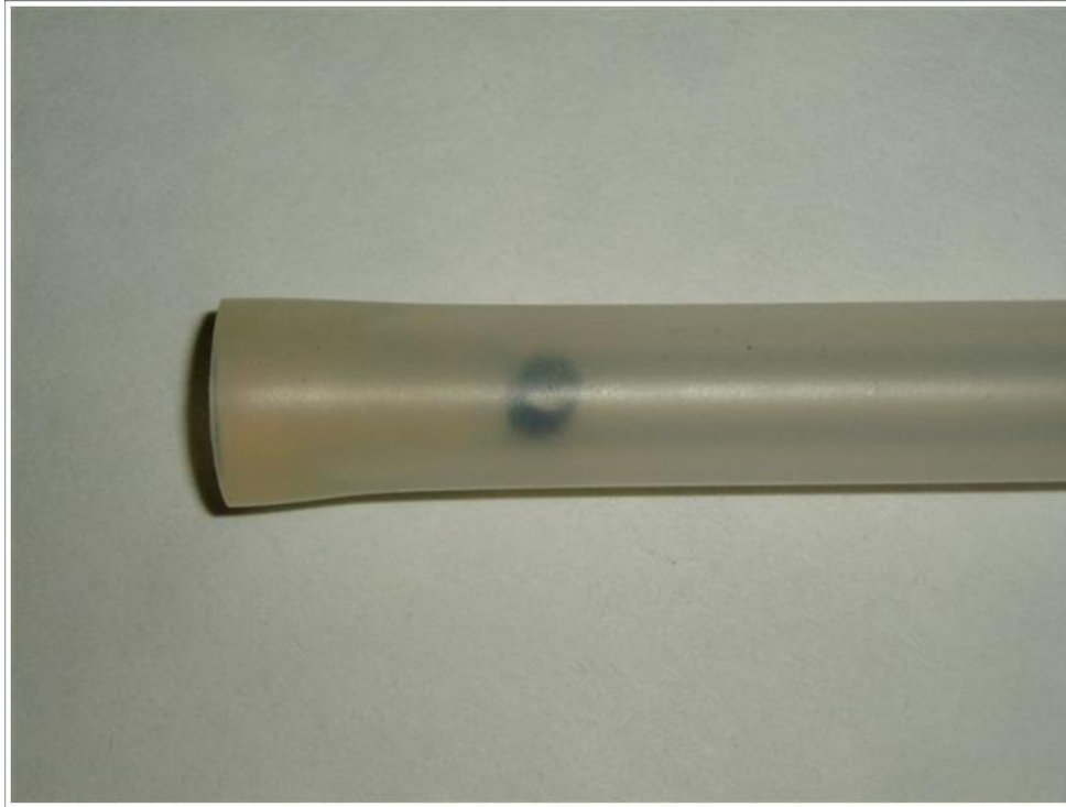
Figure 4.2: A picture of one uranium target placed inside a hose. The smaller hose carrying the nitrogen inflow is not visible.
