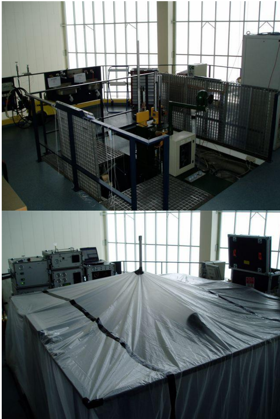
Figure 4.1: Two photos of the reactor platform: The first one without the plastic tent and the second one with the plastic tent and the SAUNA sampler in the background.
