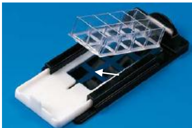
Fig. 4 | Chamber slides with gasket removal supply. We used 8-well chamber slides to culture and directly stain isolated single cells. The picture illustrates the removal of the media chambers that allows subsequent fixation and direct staining of adherent cells on the remaining microscope slide. The arrow depicts the gaps between the culture chambers. (picture adopted from Nalgene/NUNC (174) )
