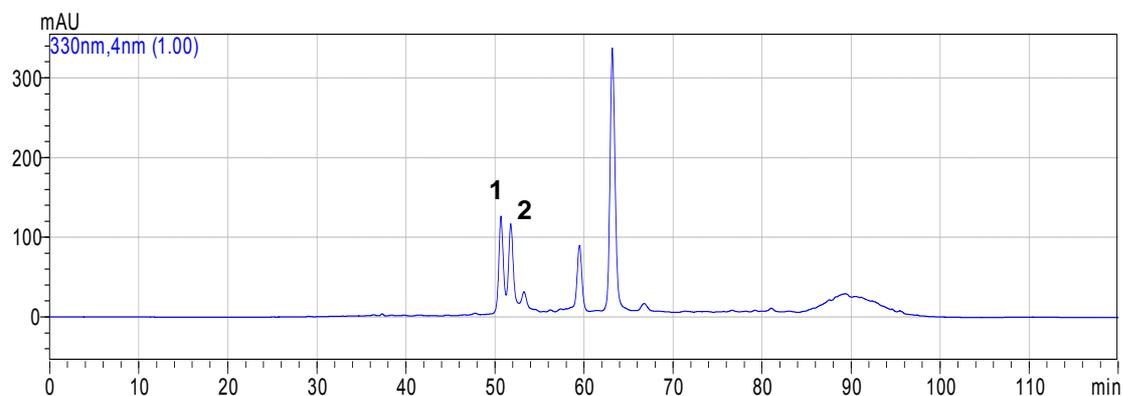
**Fig. 20** HPLC analysis of the fraction “residue” (Fig. 7, chapter 2.2.3, p. 23 and publication 2 [22] chapter 3.1. p. 30-85) on Aquasil<sup>®</sup> C 18 applying the following linear gradient: 0→10% B within 20 min, 10→20% within 60 min, 20→40% B within 20 min, 40→95% B within 10 min at a flow rate of 1 mL/min and a column oven temperature of 25°C; detected at 330 nm;
