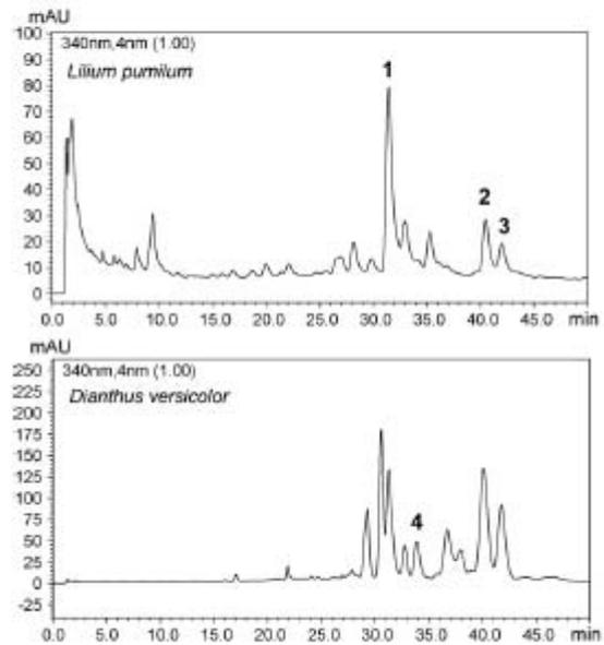
**Fig. 3.** Aqueous extracts of *Lilium pumilum* and *Dianthus versicolor* after LC-DAD-MS analysis detected at 340 nm (peak numbers correspond to structures given in Fig. 4). Deprotonated molecular ions  $[\text{M}-\text{H}]^-$ :  $m/z$  609 (1),  $m/z$  593 (2),  $m/z$  623 (3),  $m/z$  593 (4).
