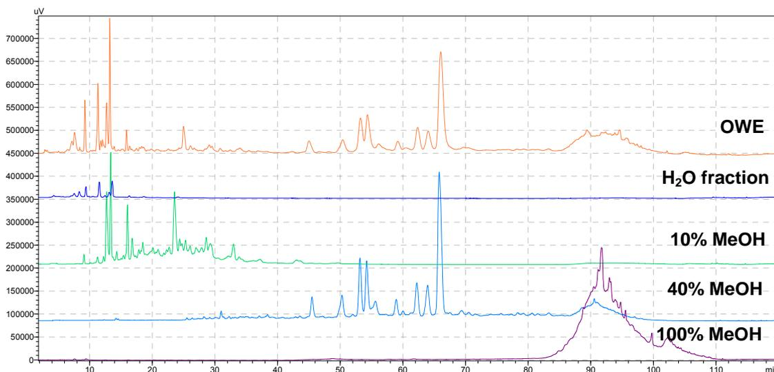
**Fig. 19** HPLC analysis of the OWE (chapter 2.2.1, p. 19) and fractions thereof obtained by SPE (chapter 2.2.2, p. 20) on Aquasil® C 18 applying the following linear gradient: 0→10% B within 20 min, 10→20% within 60 min, 20→40% B within 20 min, 40→95% B within 10 min at a flow rate of 1 mL/min and a column oven temperature of 25°C; detected at 340 nm
