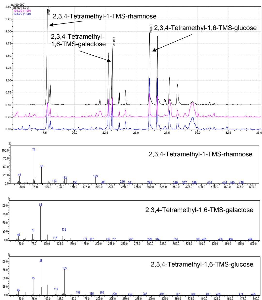
**Fig. 30** GC-MS analysis of compounds **1+2**, treated according to the method described in chapter 2.3.3, p. 25 showing EIC (upper panel) and the EI-MS spectra of the compounds eluting at 17.8 min, 22.7 min, and 26.1 min (lower panels)
