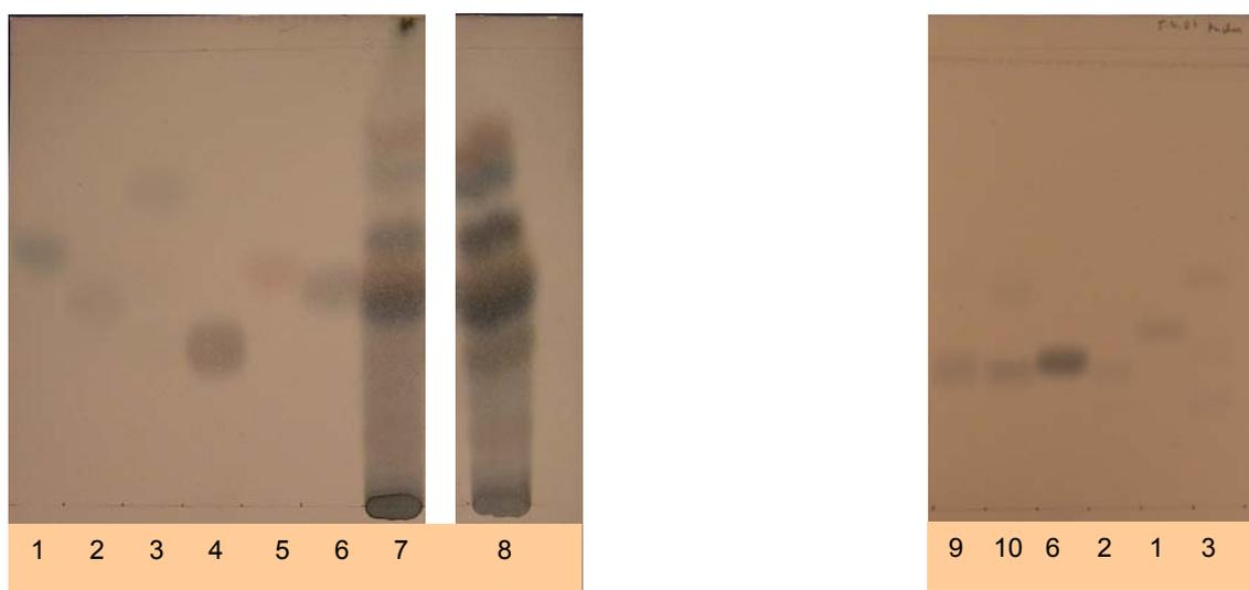
**Fig. 13a (left)** TLC analysis of the OWE (chapter 2.2.1, p. 19) of sample **a** (7) and the aqueous fraction obtained by SPE (8) in comparison to the reference substances arabinose (1), galactose (2), rhamnose (3), saccharose (4), fructose (5), and glucose (6) applying system 3 (chapter 2.3.1 p. 24, table 3) detected with diphenylamine-aniline-reagent after heating to 105-110°C
