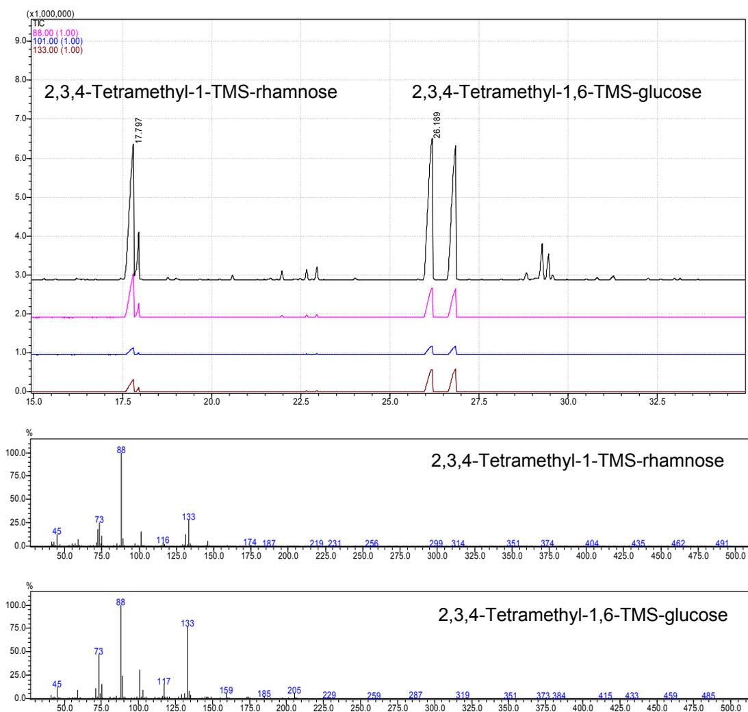
**Fig. 29** GC-MS analysis of rutoside, treated according to the method described in chapter 2.3.3, p. 25 showing the TIC and EIC (upper panel) and the EI-MS spectra of the compounds eluting at 17.7 min (middle panel) and 26.1 min (lower panel)
