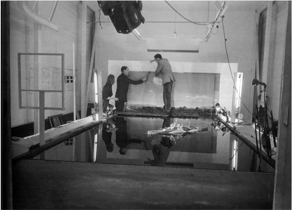
Testing the camouflage of ships at British Naval Research Laboratory at Leamington Spa.
