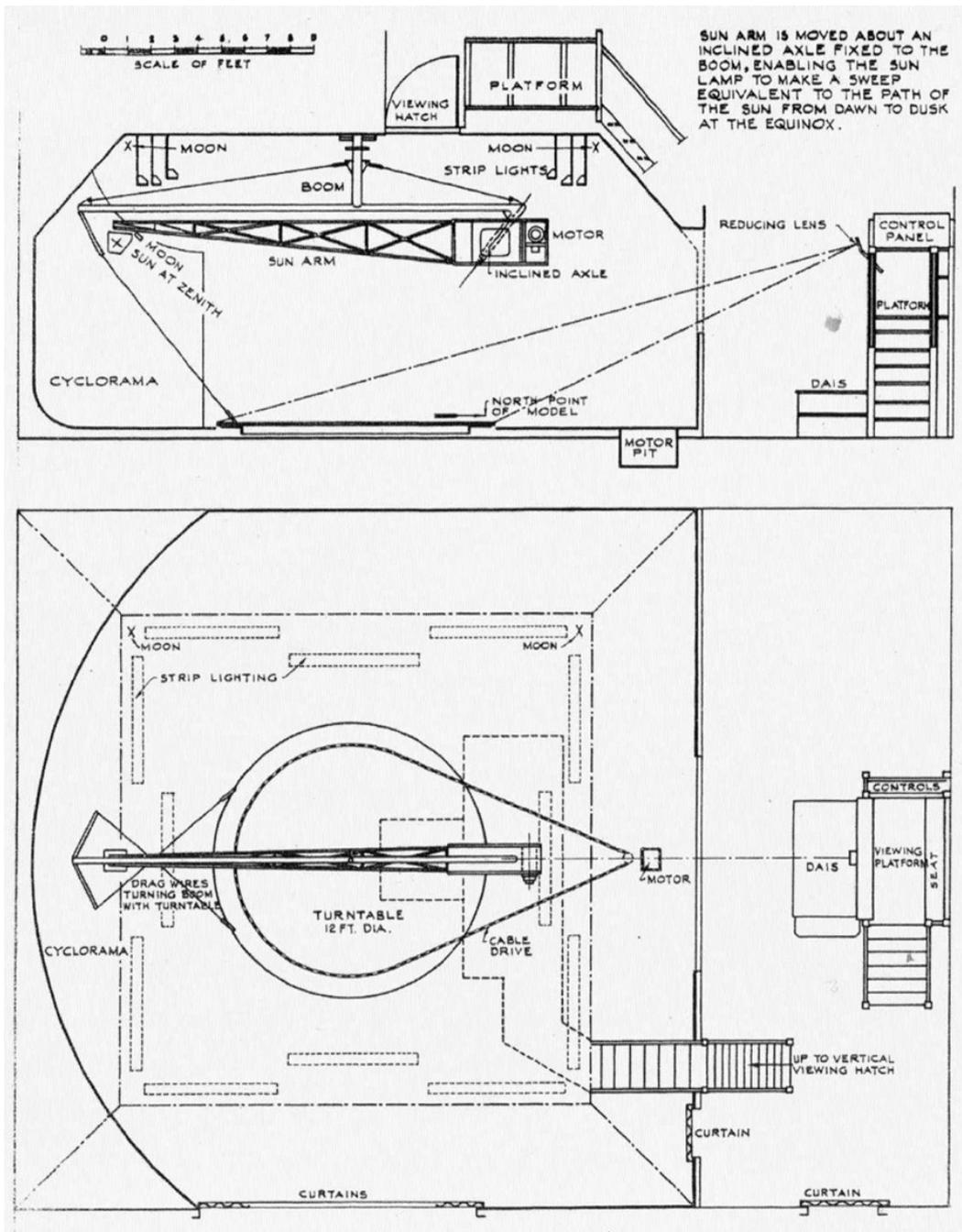
Diagram showing how the 'viewing room' at Leamington operated.
