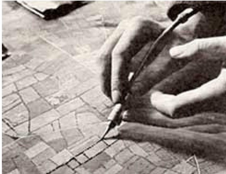
Applying hedges to a terrain model using a compressed extrusion gun.
