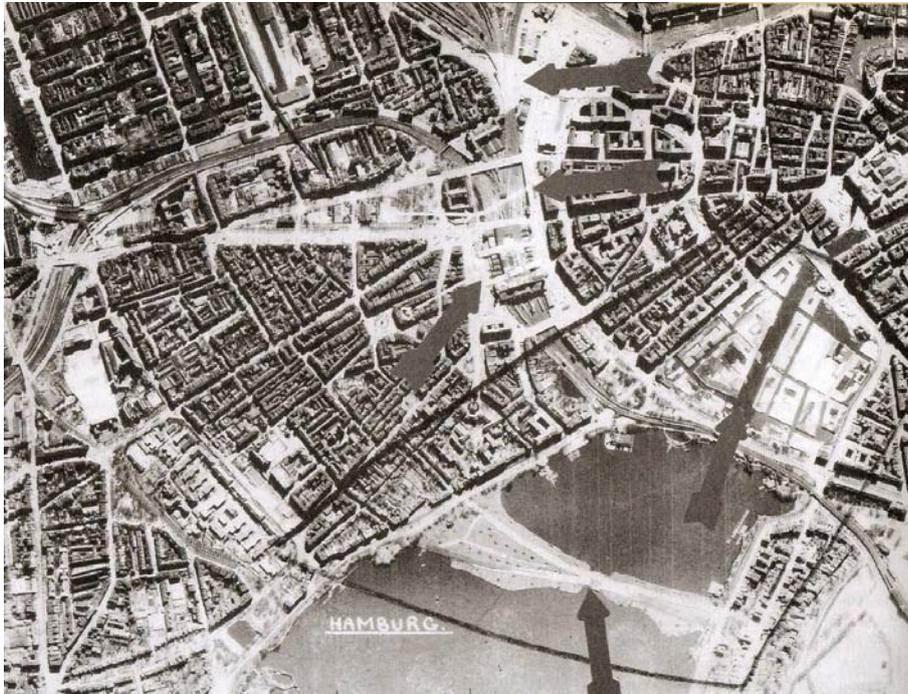
Hamburg's camouflage project caught under construction by RAF photoreconnaissance, 8 April 1941. The upper three arrows show paintwork designed to disguise railway patterns. Arrows at lower right show the decoy Lombards Bridge and covered-over Binnen Alster.
