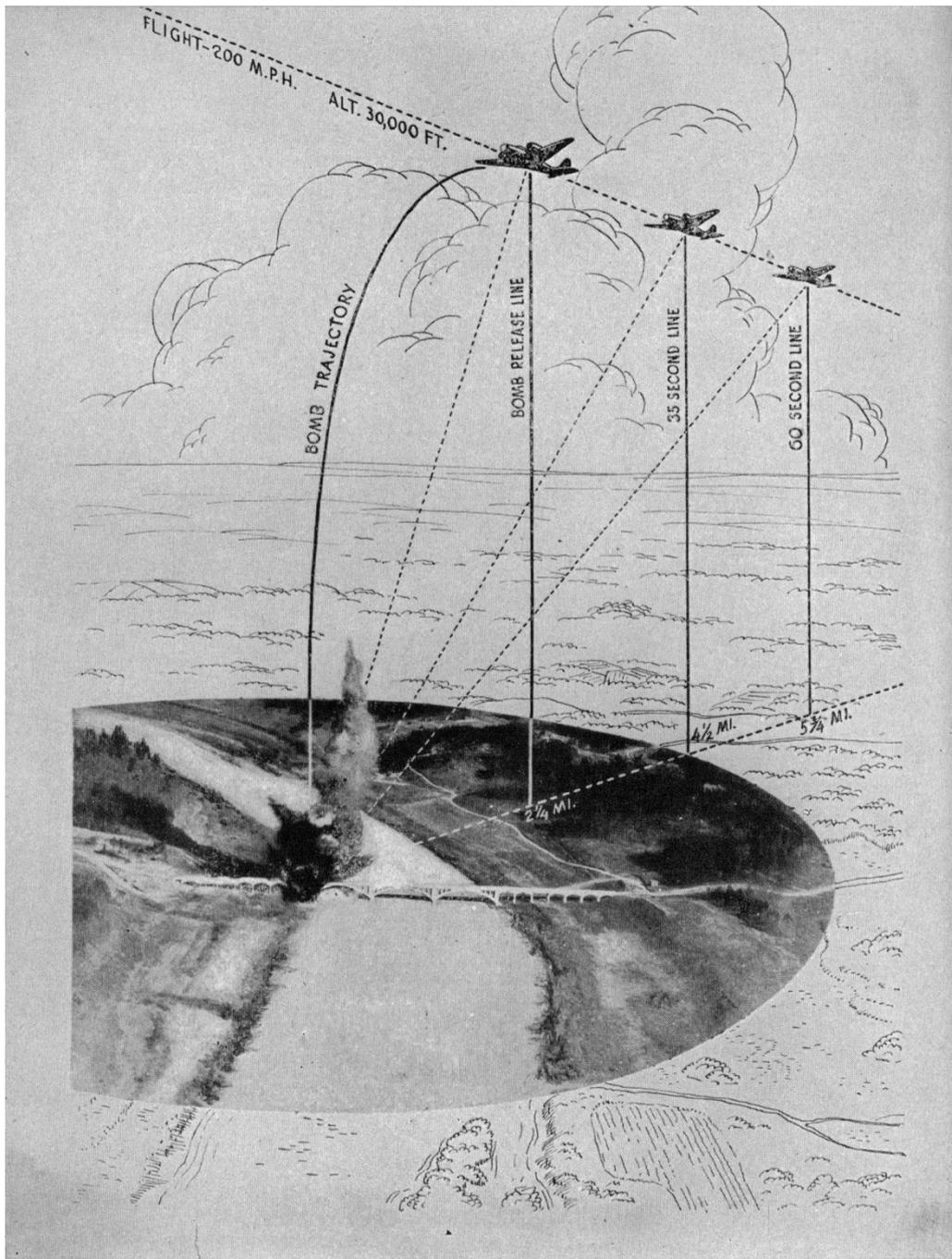
'Precision bombing diagram. Bombardier must see the target and have bomb sight in operation at 35-second line for precision bombing. Greater accuracy is possible if target can be seen from the 60-second line.' (Robert Breckenridge, 1942)
