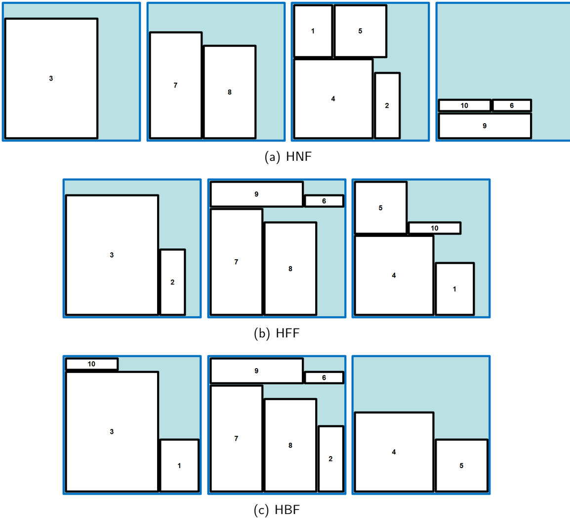
Figure 2: Two-phase level packing algorithms
