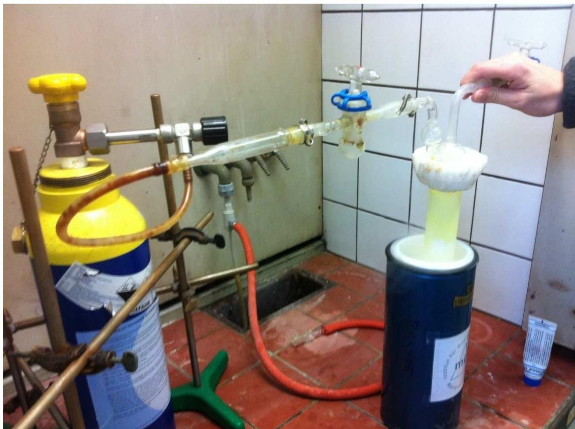
*Fig. 3.7 Transfer of chlorine gas into a cooling trap under the exhaust hood*
