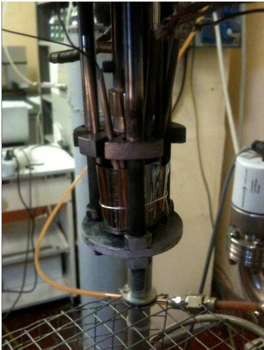
*Fig. 2.4 Knudsen cell-like holder with a “sandwich-type” arrangement for the electrodes and the electrolyte [photo: Virgilio Genova]*
