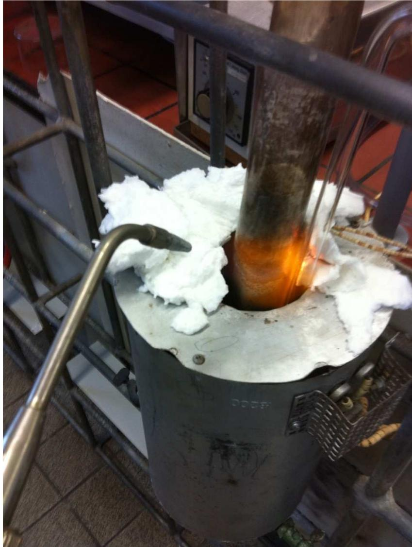
*Fig. 3.10 Melting down the condensed parts of the electrolyte with a hydrogen torch*
