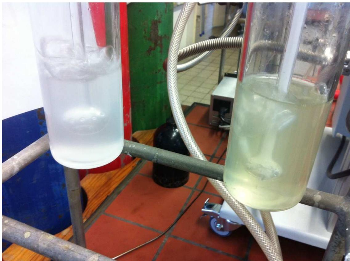
*Fig. 3.9 Chlorine gas bubbling through aqueous sodium hydroxide solutions. The slightly green color of the solution in the right bottle shows the presence of dissolved chlorine*
