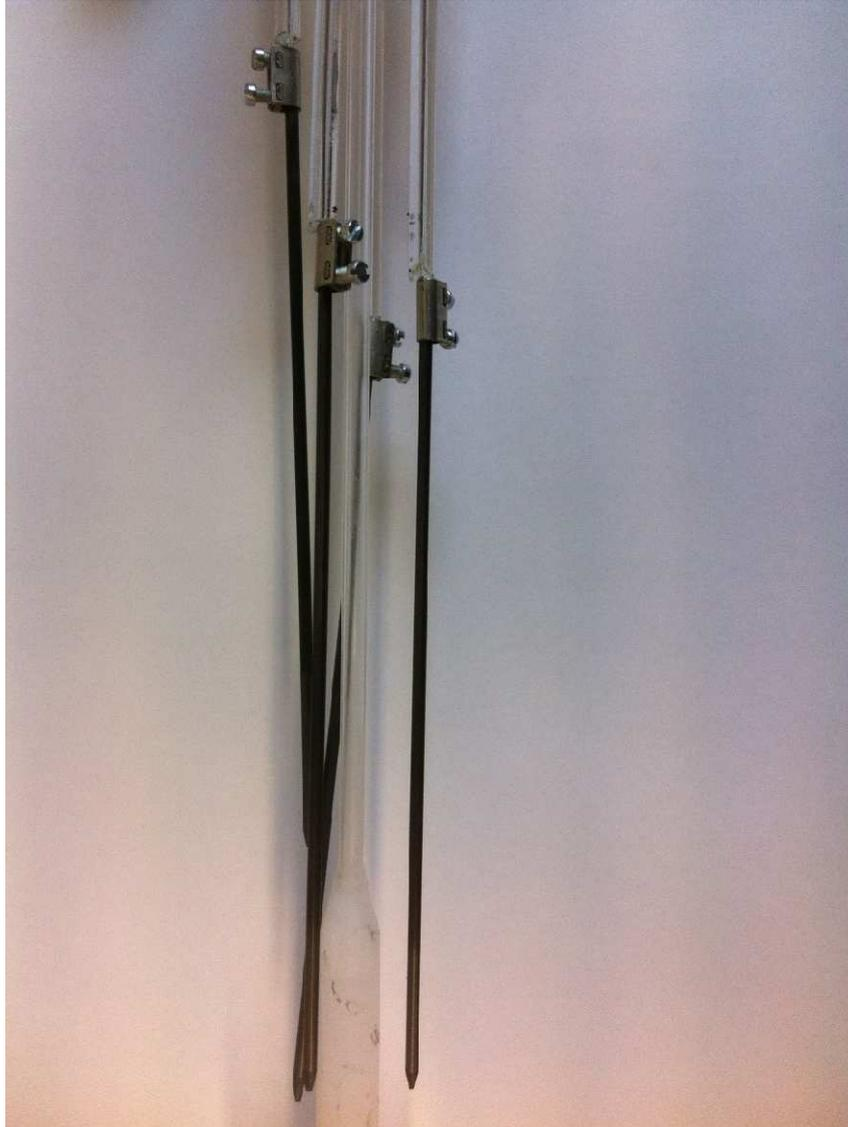
*Fig. 3.14 Graphite rods at the end of the molybdenum lead wires to prevent interactions between the Mo and the investigated alloys*
