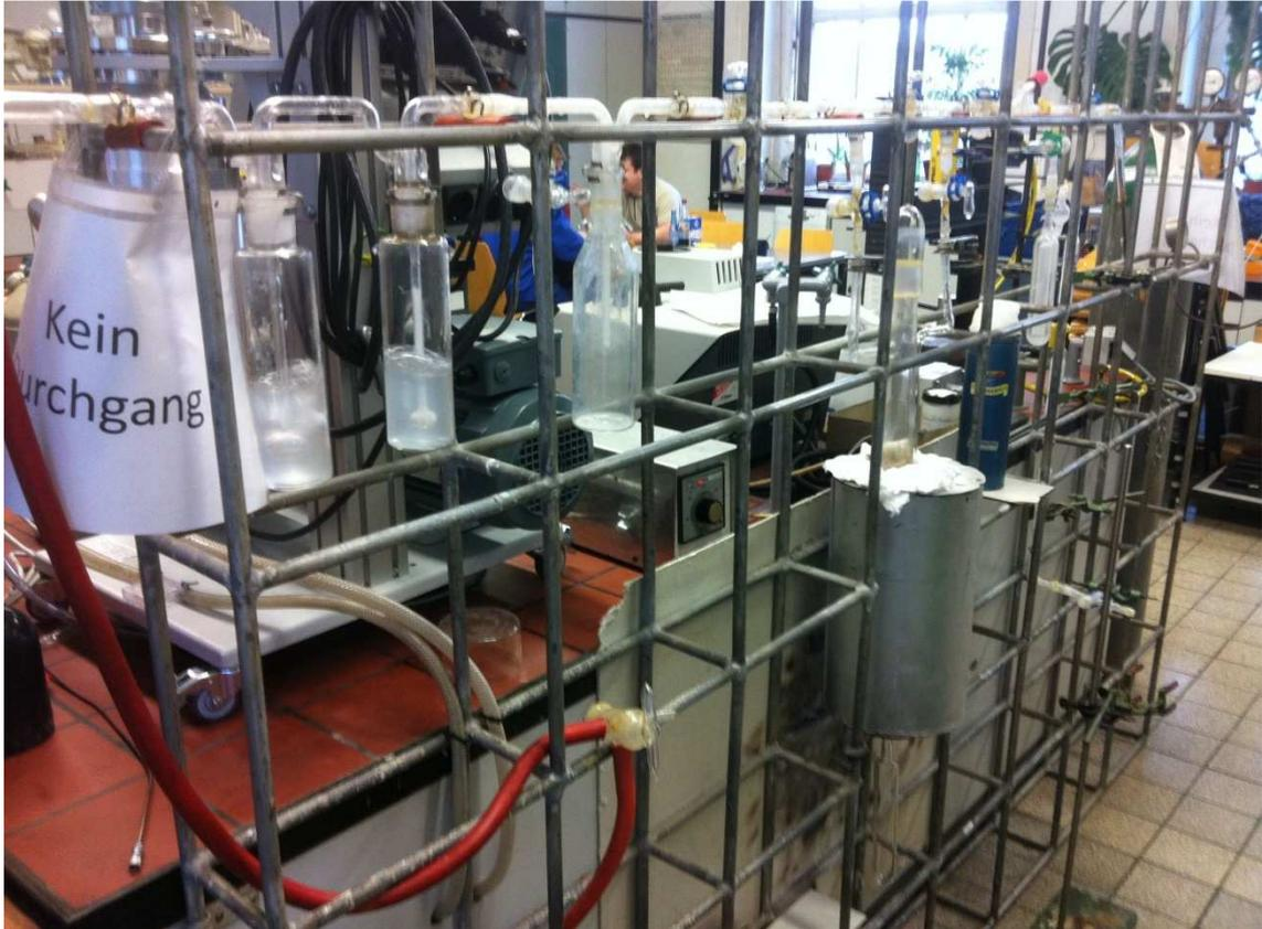
*Fig. 3.6 The apparatus for the preparation of the  $KCl-LiCl-KAlCl_4$  electrolyte*
