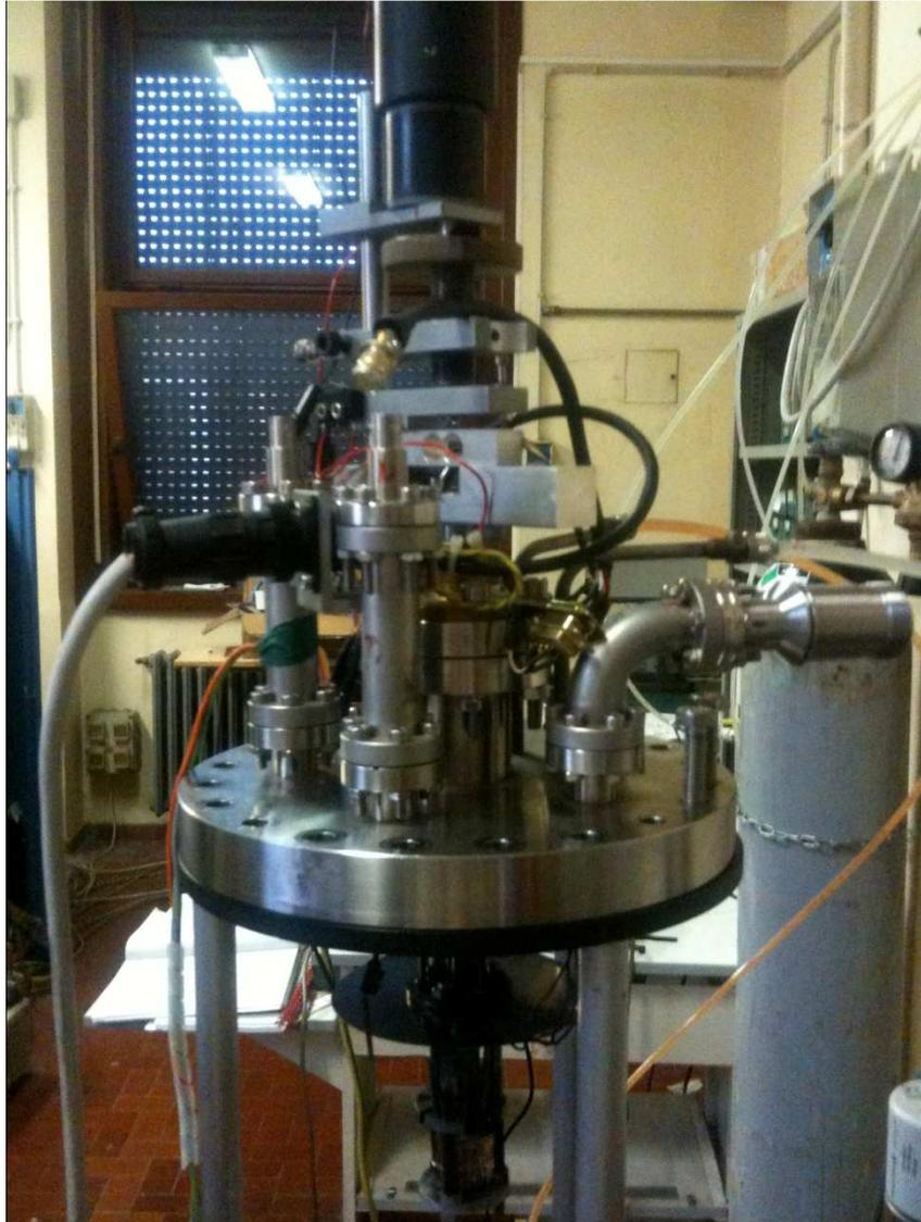
*Fig. 2.6 Feedback-motion device for the compensation of size changes of the electrodes and the electrolyte due to the high temperatures [photo: Virgilio Genova]*
