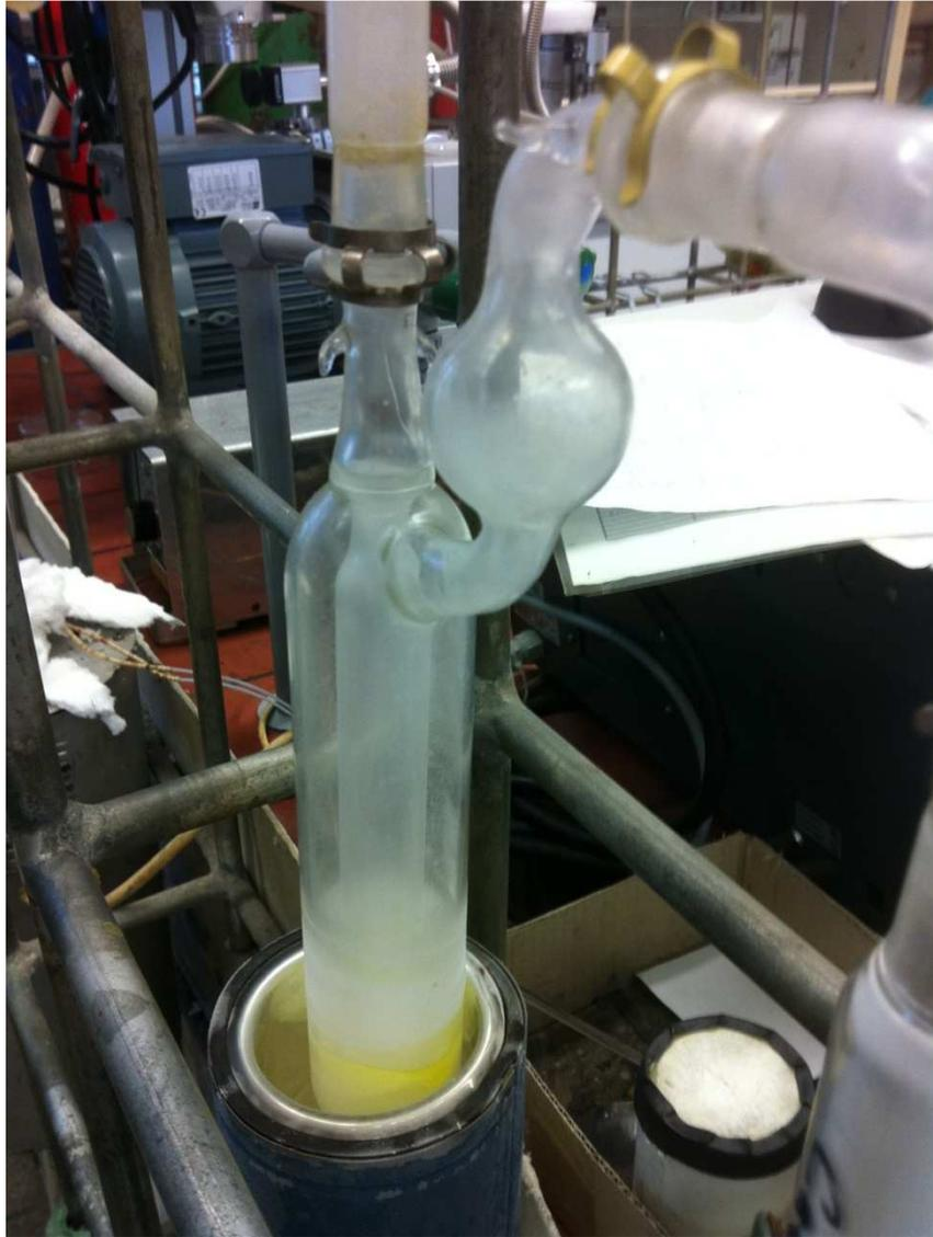
*Fig. 3.8 Chlorine gas inside of the purification-apparatus*
