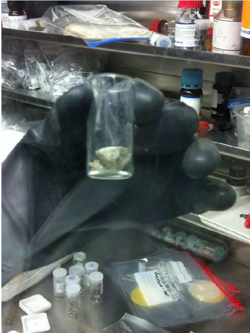
*Fig. 3.5 Handling of moisture sensitive  $KAlCl_4$  inside of the glovebox*
