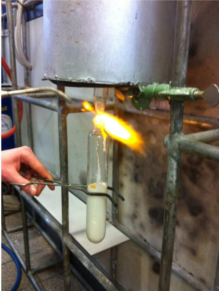
*Fig. 3.11 Sealing the purified electrolyte into an ampoule
