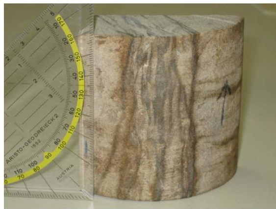
Figure 5: Core sample with deformation bands, 1651 m.
