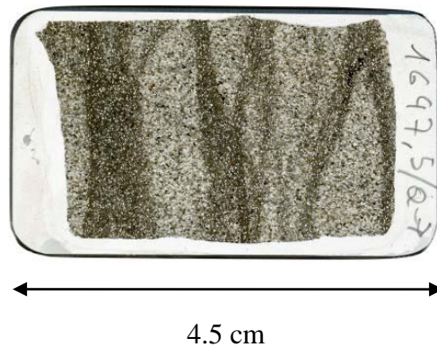
Figure 6: Thin-section scan of the sample 1647.5m. Deformation bands are clearly visible as dark, anastomosing bands of 3-10 mm thickness.
