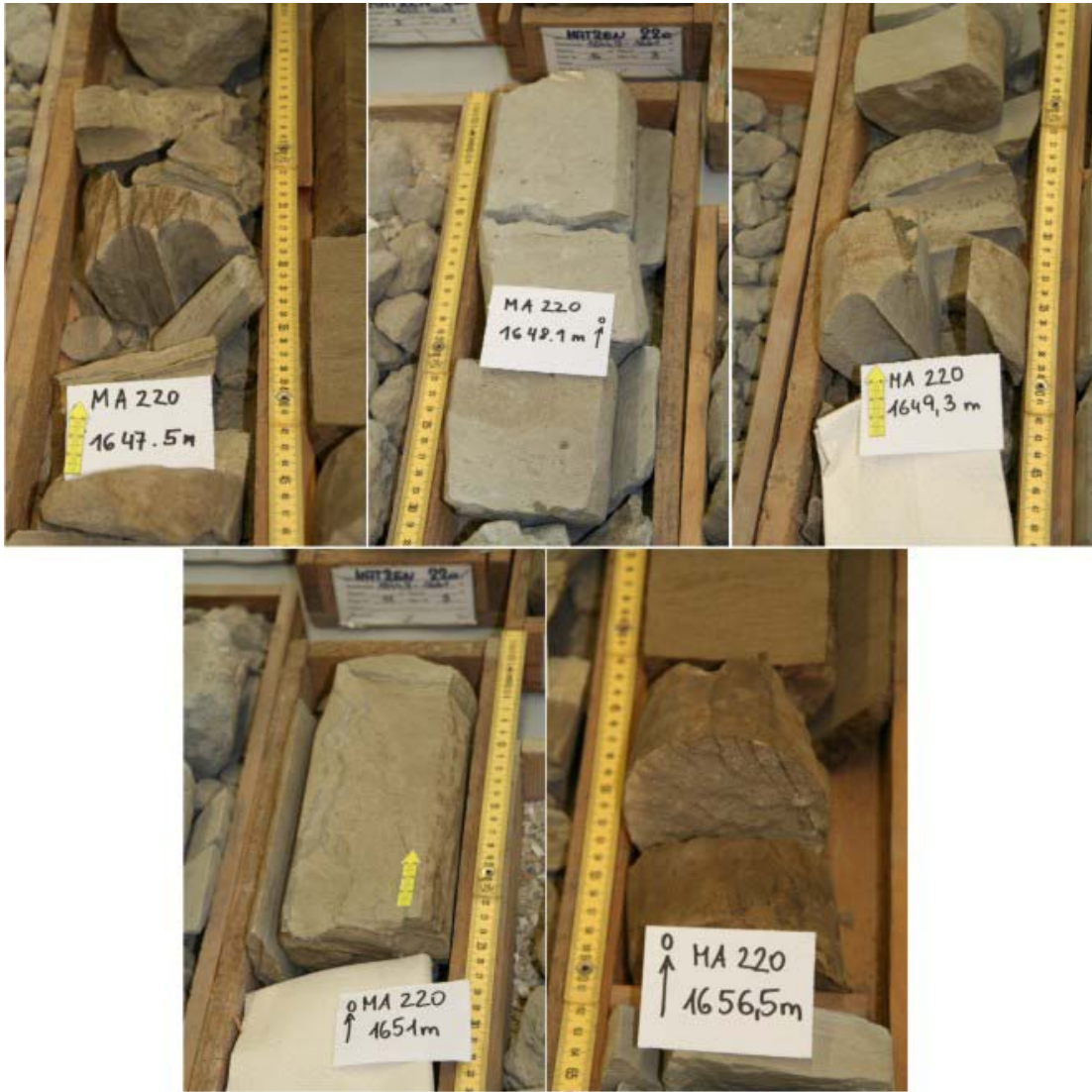
Figure 4: The five core samples from Matzen 220 analyzed in this study. Note the oil staining in the lower right image.
