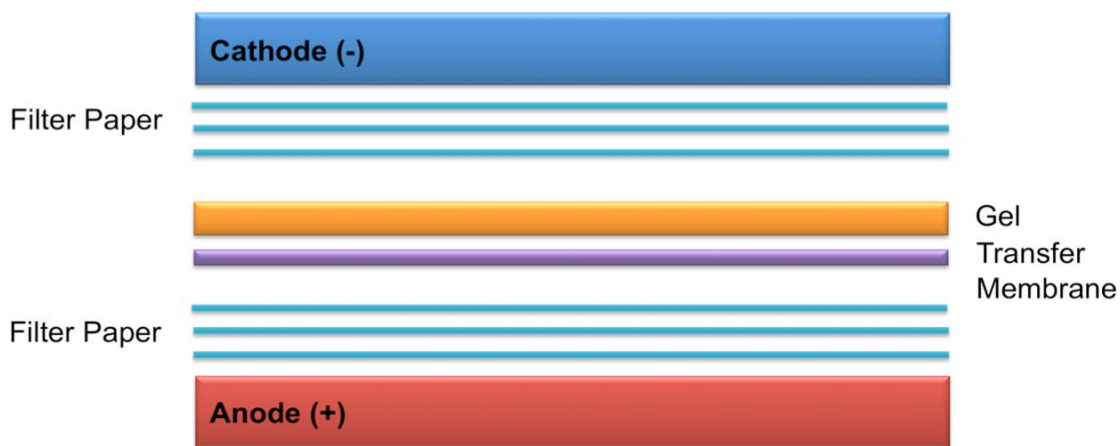
Fig. 13 Sandwich assembly of a semi-dry blot
