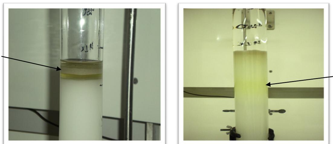
Figure 10. Column with the added Cal1L1 oil. Figure 11. Separation of the Cal1L1 oil in the column, with the arrow pointing at the yellow-coloured band.
