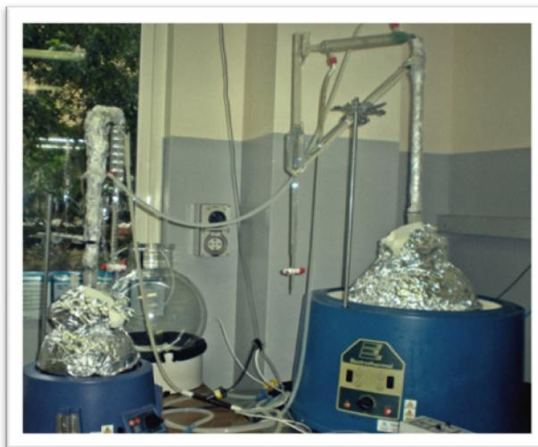
Figure 7. Water steam distillation apparatus.
