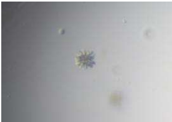
Figure 27. GTPase domain-Ged fusion protein crystals. A. Initial hit observed after 1 day in 0,1 M sodium citrate pH 5,5 20 % (w/v) PEG 3000. B. Initial hit in 0,2 M lithium sulfate, 0,1 M Bis-Tris pH 5.5, 25 % (w/v) PEG 3350 after 11 days. 10,4 mg/mL monomeric protein was used.
