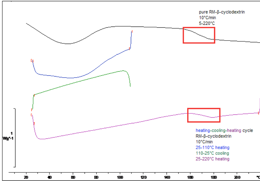
Figure 17: DSC thermograms of pure RM \beta CD and also its heating-cooling-heating cycle in the colors blue, green and violet. The red box indicates the glass transition.
