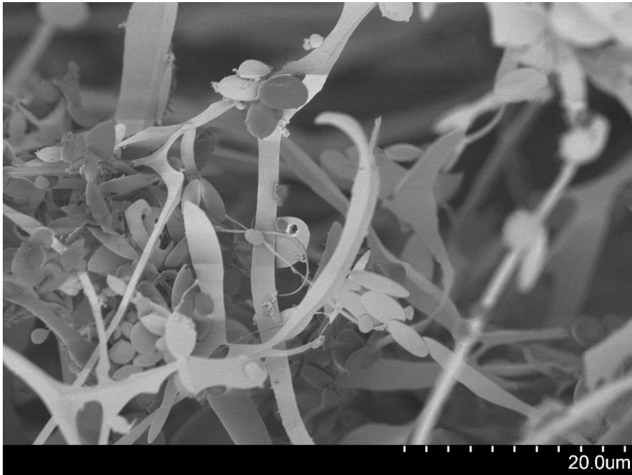
Figure 27: SEM picture of the freeze-dried curcumin/ RM \beta CD/ HPMC system with a magnification of 2200
