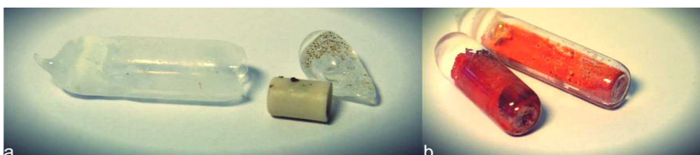
Fig. 4.8 samples that could not be used for analysis due to a) Bursting in the furnace b) Extensive evaporation of phosphorus
