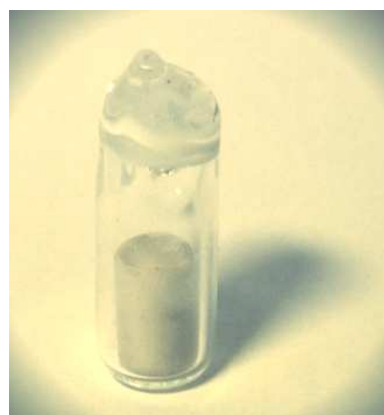
Fig. 4.7 sealed samples of Ni-P-Sn
