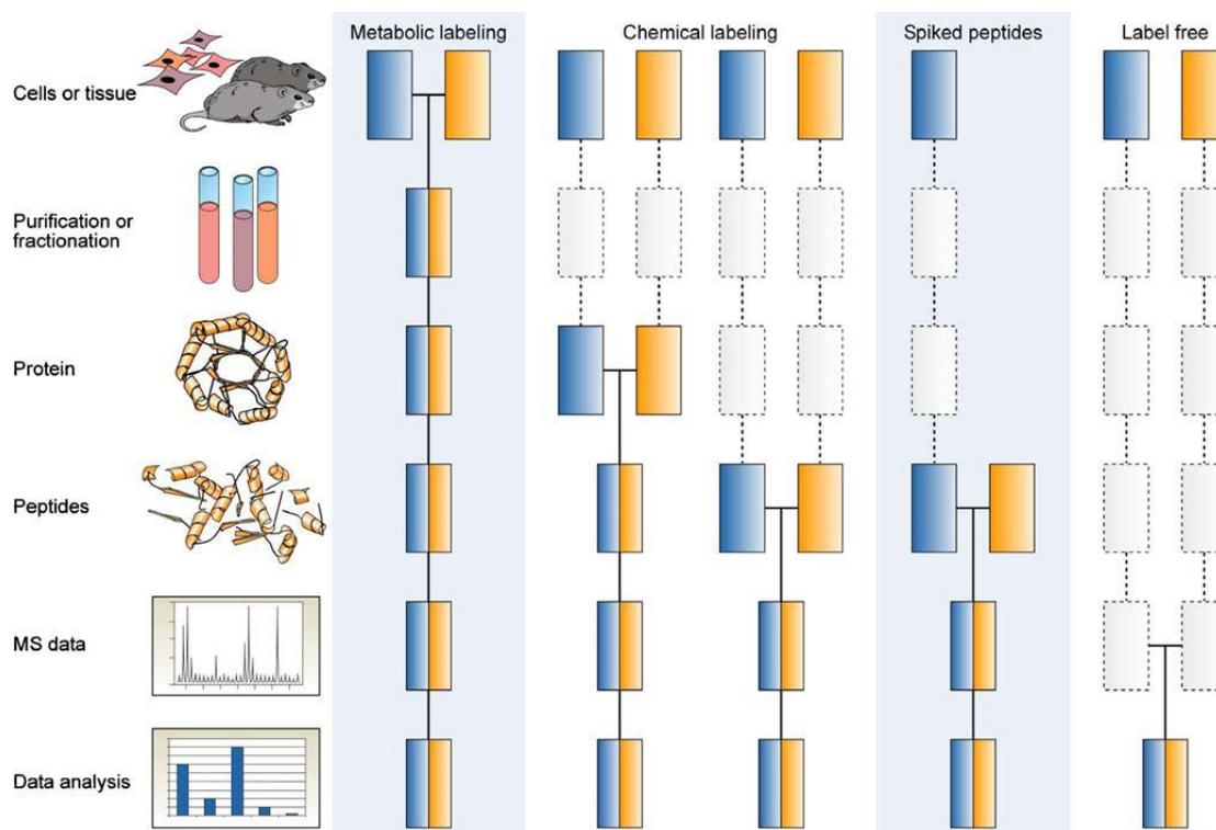
**Figure 9.** Quantitative mass spectrometry workflows introducing heavy/light isotope-codes at different stages of the sample pretreatment. Boxes in blue and yellow represent two experimental conditions. Horizontal lines indicate when samples are combined. Dashed lines indicate points at which experimental variation and thus quantification errors can occur, (taken from (Bantscheff et al., 2007)).
