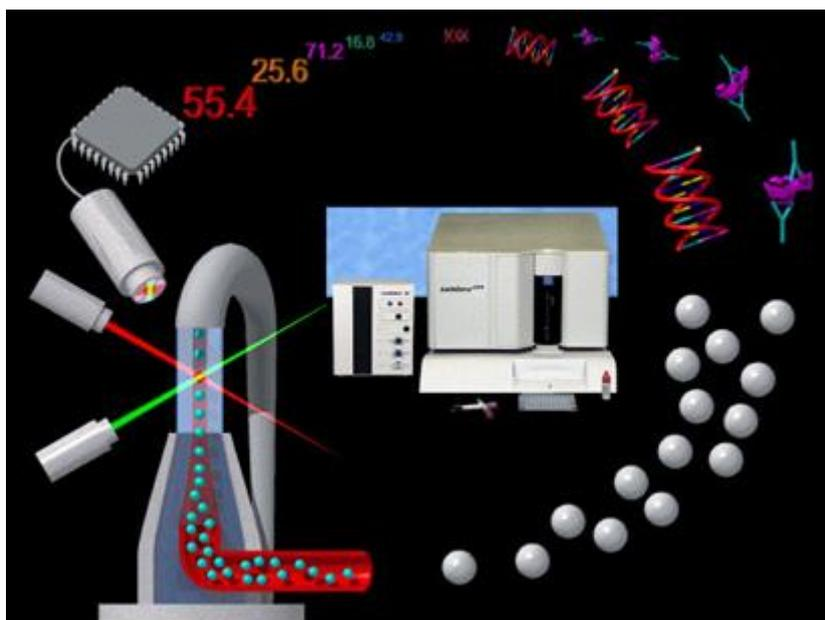
**Figure 2.** Main parts of Luminex™ System: biomolecules; microspheres (beads); flow analyzer and high-speed signal processing, (taken from (Dunbar & Vander Zee & Oliver & Karem & Jacobson, 2003)).
