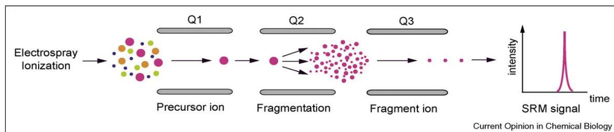
**Figure 14.** Schematic illustration of the principle of Selected Reaction Monitoring (SRM): Q1- precursor ion isolation; Q2- precursor ion fragmentation; Q3- mass analysis and quantification of a specific precursor ion fragment (transition), (taken from (Huttenhain& Malmstrom& Picotti& Aebersold, 2009)).
