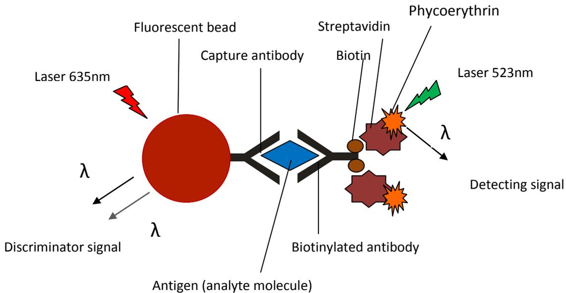
**Figure 1.** Schematic drawing of a Luminex assay.
