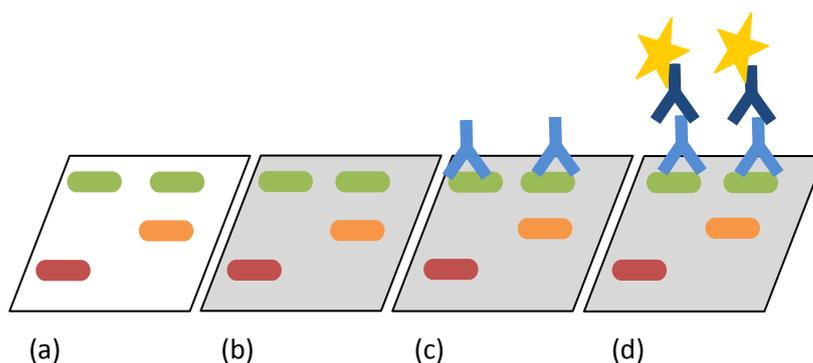
**Figure 7.** Consecutive steps in membrane “development”: (a) membrane after protein transfer; (b) blocking the membrane on the sites not occupied by transferred proteins; (c) incubation with primary antibodies; (d) incubation with enzyme-linked secondary antibody and the color-reagent (chemiluminescence) solution.
