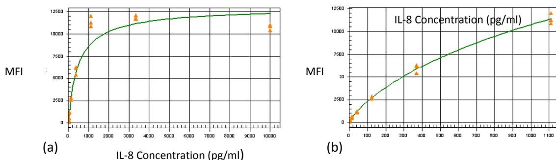
**Figure 32.** Standard calibration curves of Luminex™: (a) curve covering the entire concentration range of IL-8 standards; (b) standard curve in the concentration range < 1111pg/ml. The series of standard concentrations were made using Luminex buffer.
