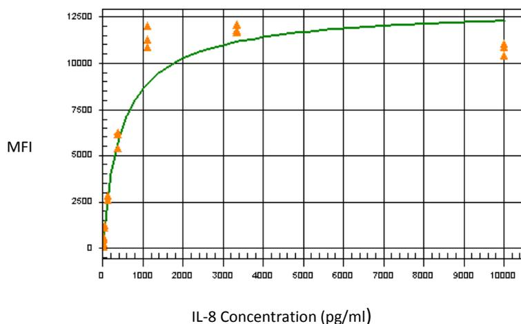
**Figure 3.** Example of MFI response in dependence on analyte concentration: Experimental data are given by orange triangles; fitted curve based on eqn. 1 is given as green line. This curve is a typical output of the instrument's "data interpretation report".
