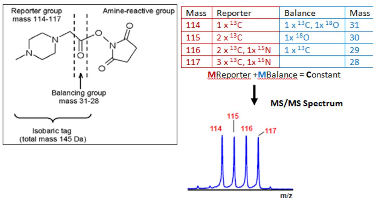
**Figure 12.** Left side: iTRAQ label consisting of isobaric tag and reactive group; right side: Table giving the isotope composition of four isobaric tags; and typical MS/MS spectrum showing the reporter-group section, (taken from (Ross et al., 2004)).
