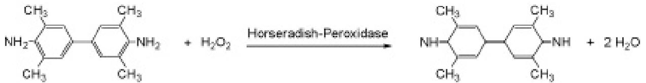
**Figure 5.** Scheme of the Horseradish Peroxidase reaction.
