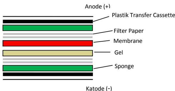
**Figure 6.** Scheme of the various layers used during the blotting process in WBAs.
