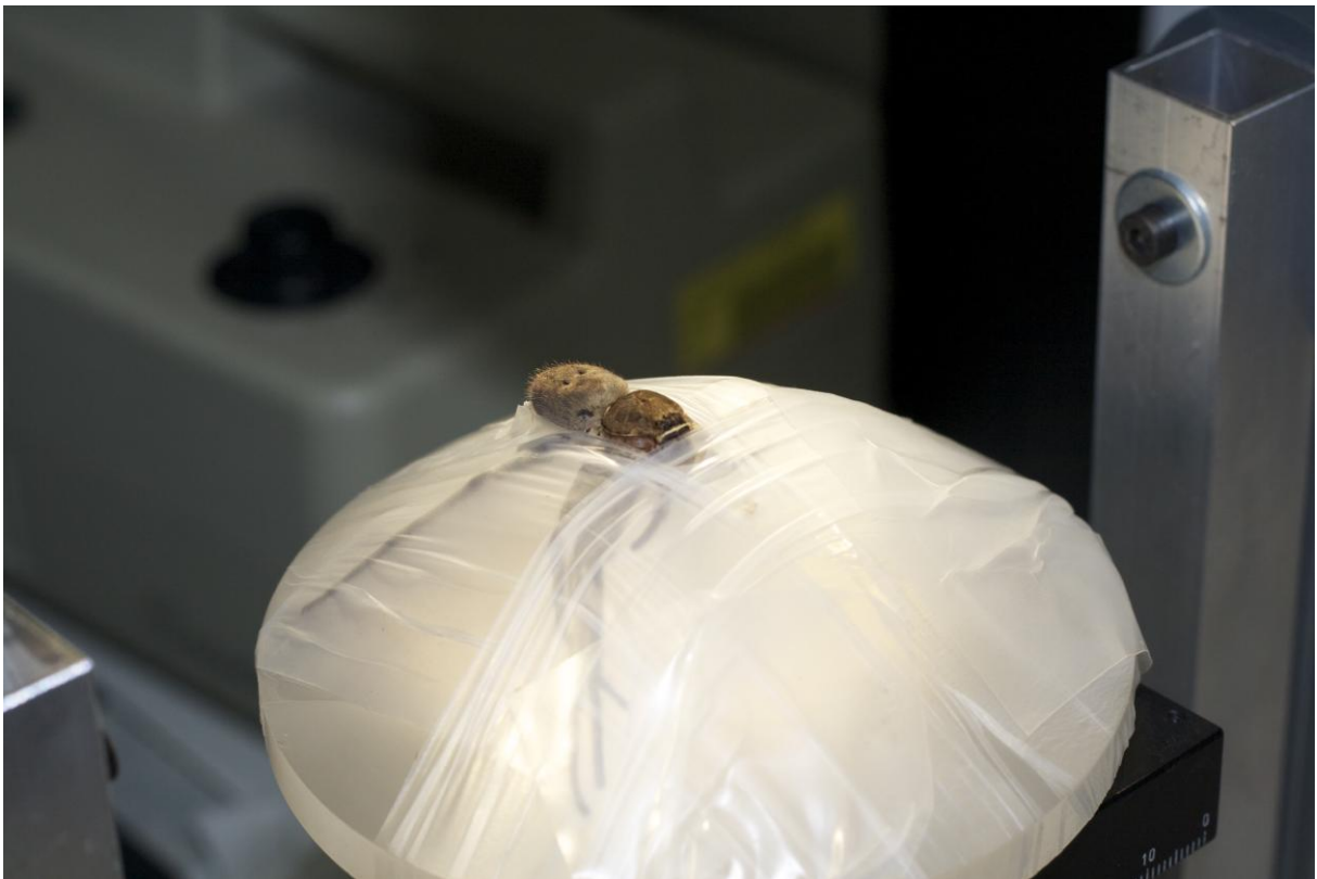
Fig. 13: Heteropoda venatoria (female) fixed on a plastic hemisphere and positioned in the goniometer device. Light from above illuminates the spider. A micromanipulator on which the hemisphere was installed allows moving the spider in any position needed.
