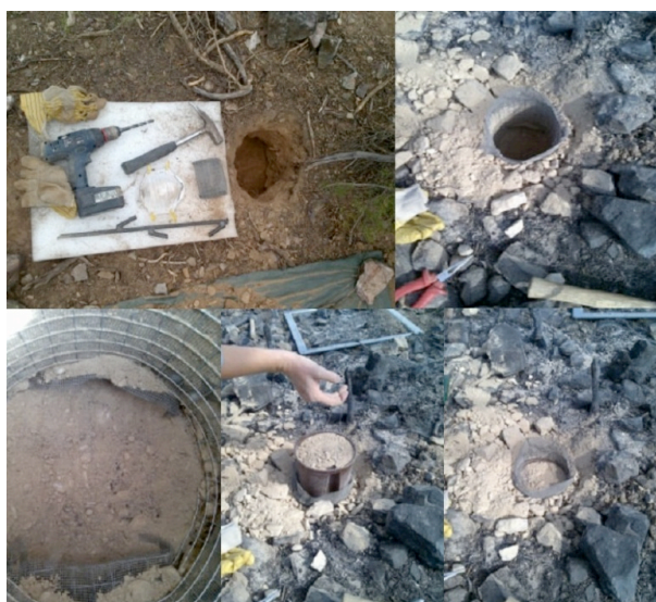
Fig. 10 – Construction of the tunnels for the resin bags. Photo: Póvoas
