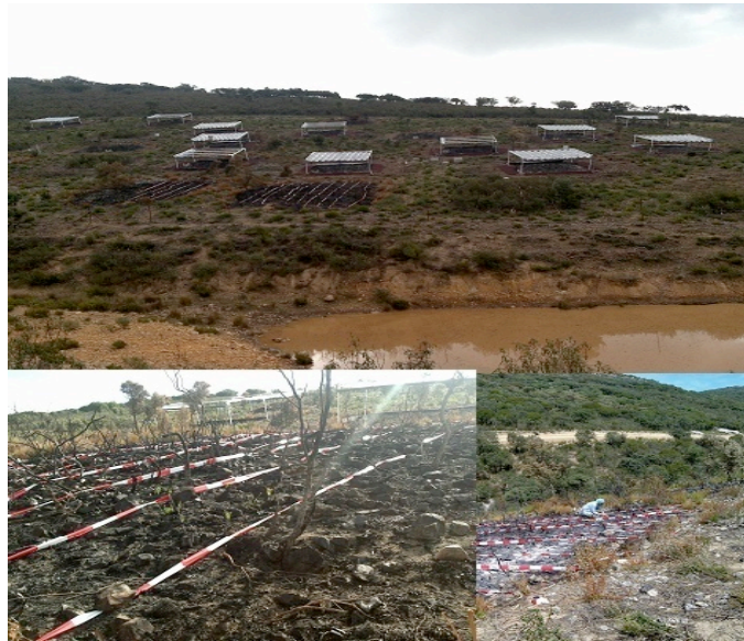
Fig. 7 – Plots from the study area. Control, burned and roofed plots and the grid sampling scheme for soil sampling. Photo: Póvoas
