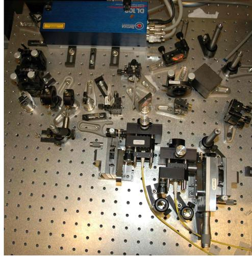
**Fig. 4.2:** Photograph of the Sagnac source used for the presented experiments.
