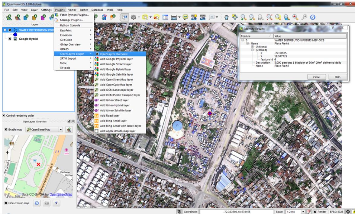
Figure 14: Screenshot of *Quantum GIS* showing the *OpenLayers* plugin in combination with a water distribution point layer
