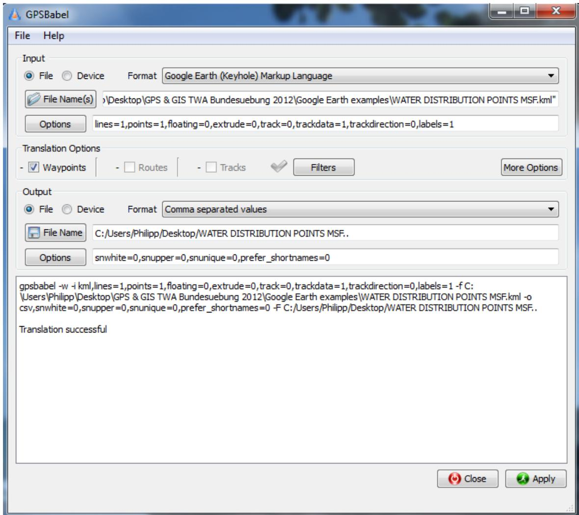
Figure 11: Screenshot of *GPSBabel* showing the conversion of a *Google Earth* layer with water distribution points to a spreadsheet file for print or further processing
