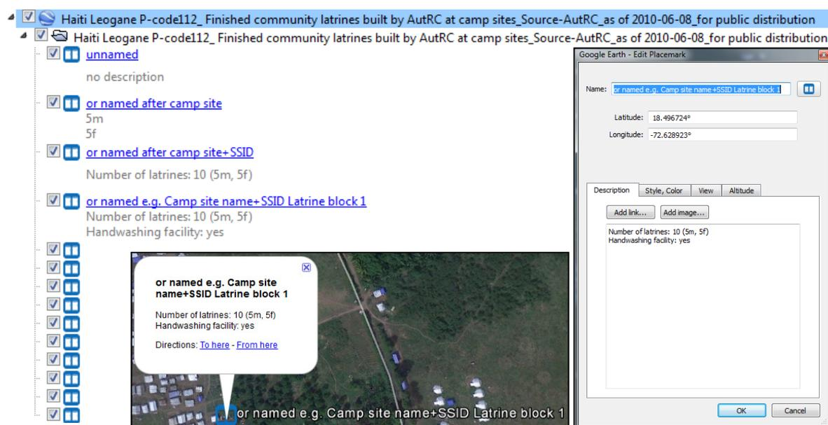
Figure 26: Data structure example of a *kml/kmz* file in *Google Earth*
