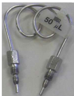
Fig. 4.8. Sample loop with 50 \mu l volume.
