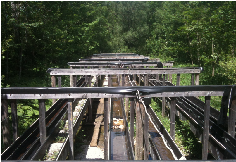
Figure 1 Flumes where heterotrophic biofilms were grown and fed with stream water from the Oberer Seebach, Austria
