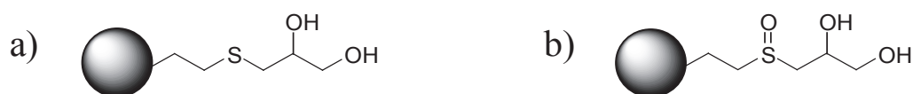
Fig. 19: The chemical structure of a) non-oxidized thioglycerol phase (TG) b) oxidized thioglycerol phase TGO (respectively SGO in Appendix II + III).
