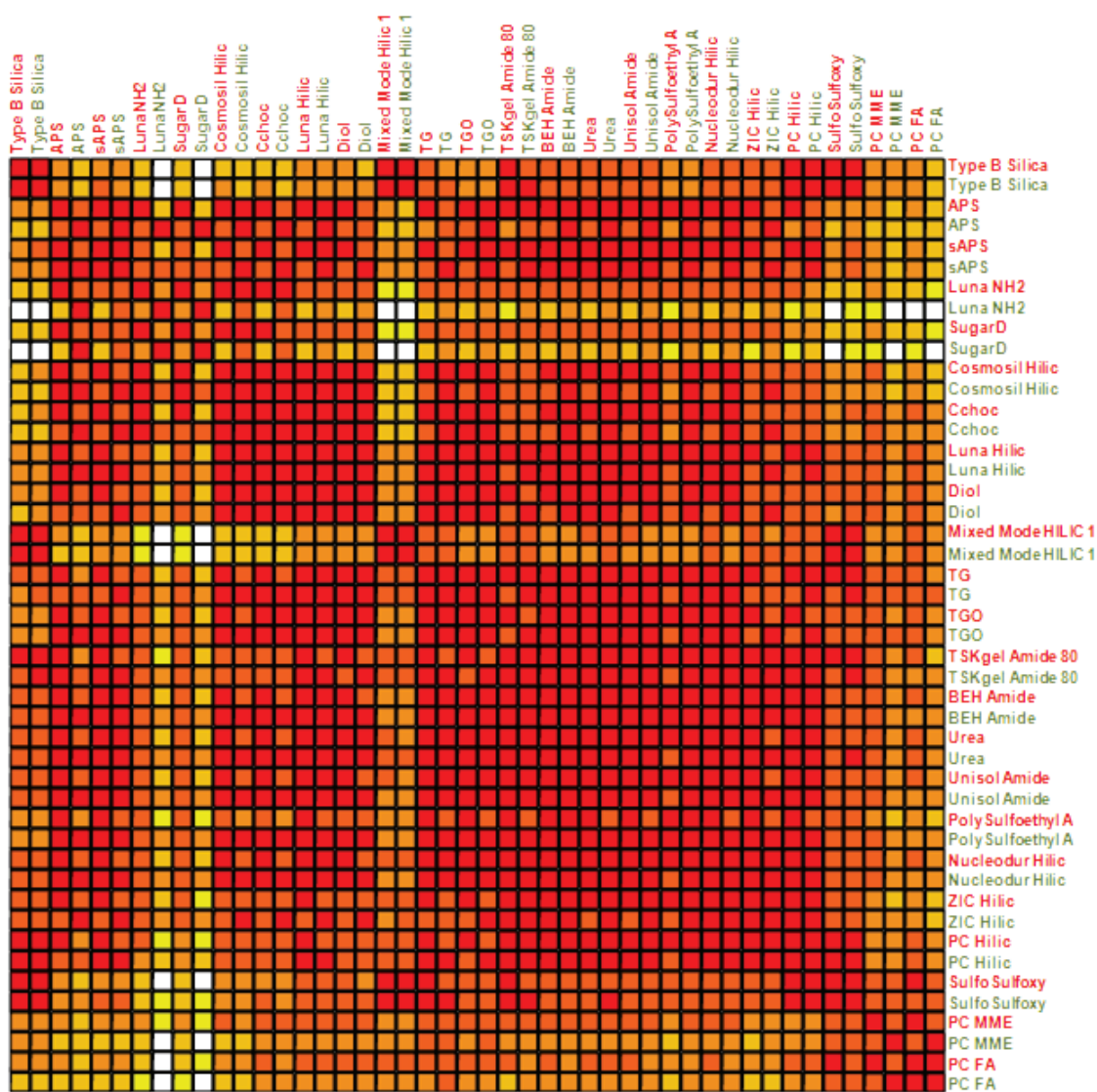
Fig. 27: Correlation matrix of screened HILIC columns. Red column labels relate to a MP condition of ACN/H 2 O (90:10, v/v) + 10 mM NH 4 FA (pH 3) while green SP labels express the analysis with ACN/H 2 O (90:10, v/v) + 10 mM NH 4 AcOH (pH 5). The color encryption of the squares is explained in the text.
