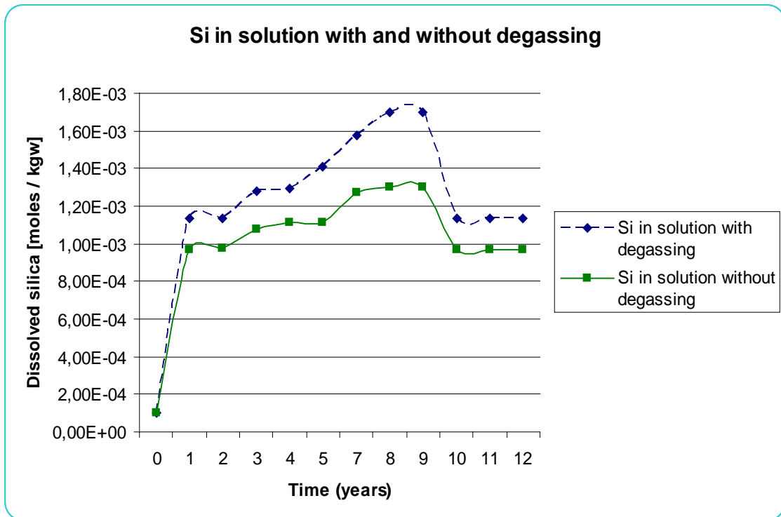
Figure 51: Results from numerical experiment 7 showing dissolved silica in solution with and without CO 2 degassing
