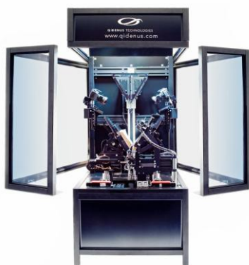
Figure 4: 2008 Model 1 Qidenus Robotic Book Scanner
