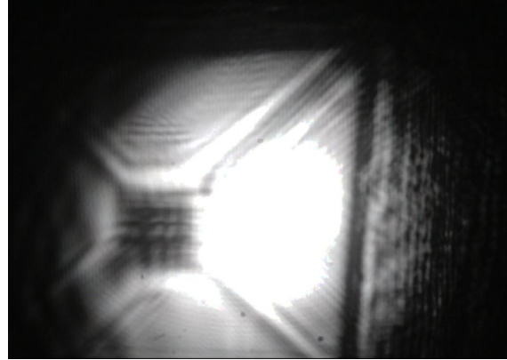
FIGURE 4.2: Photonic crystal membrane imaged by a camera. The camera was placed behind the membrane in transmission. Illuminated by the laser beam (white spot), one can see very well the clamping of the membrane and the photonic crystal area. With the help of the camera, finding the right membrane on the chip and rough beam positioning was fairly easy.
