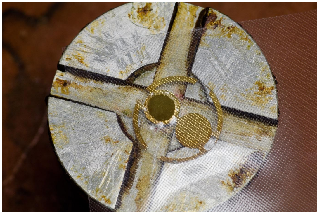
Figure 17 Spin coater with QCM mounted together with mask to coat one electrode
