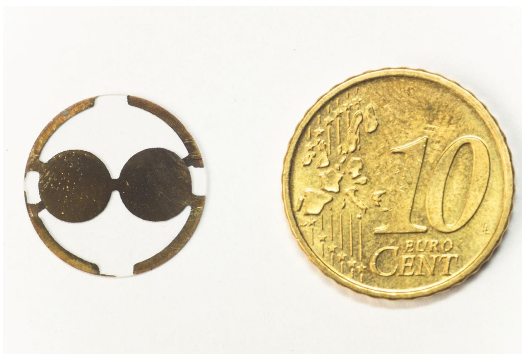
Figure 2 Image of a 10 MHz quartz crystal microbalance as applied in this thesis
