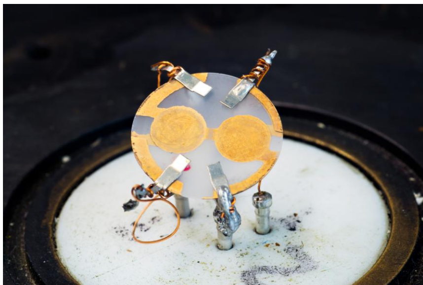
Figure 18 QCM mounted onto the custom-made oscillator circuit
