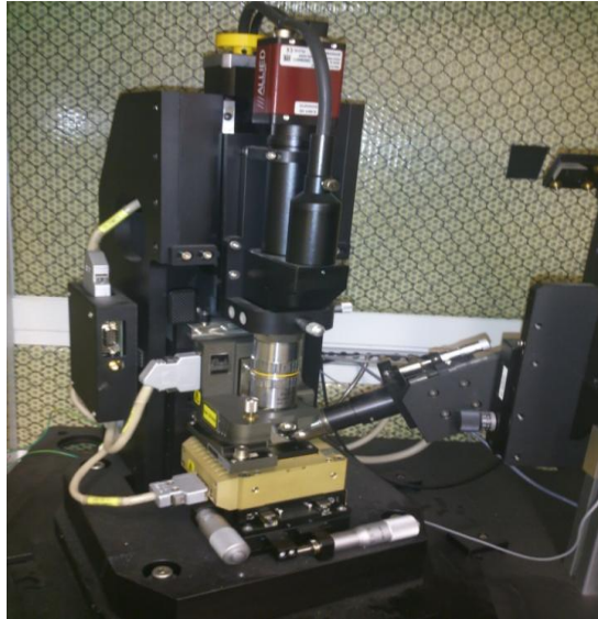
Fig. 3.4. XE 100 AFM from Park Systems The images were processed with WSxM 5.0 Developer 6.3 software. A sample AFM image of exfoliated single layer graphene is shown in the Fig. 3.5 (a) and (b).
