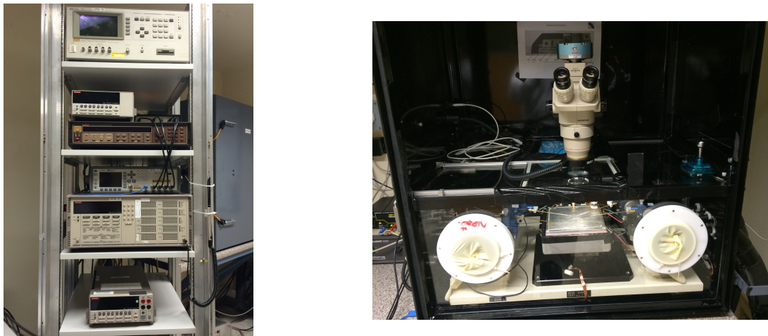
Figure 5.3: Process quality control setup. Left: Measurement Instruments, Right: Interior of the light tight box showing the vacuum support with a incorporated Peltier-Element inside a glove box.
