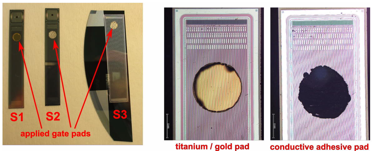
Figure 7.4: Samples with applied gate pads used for FET-like measurements. Left: All samples, right: Enlarged view of the different gate pads.
