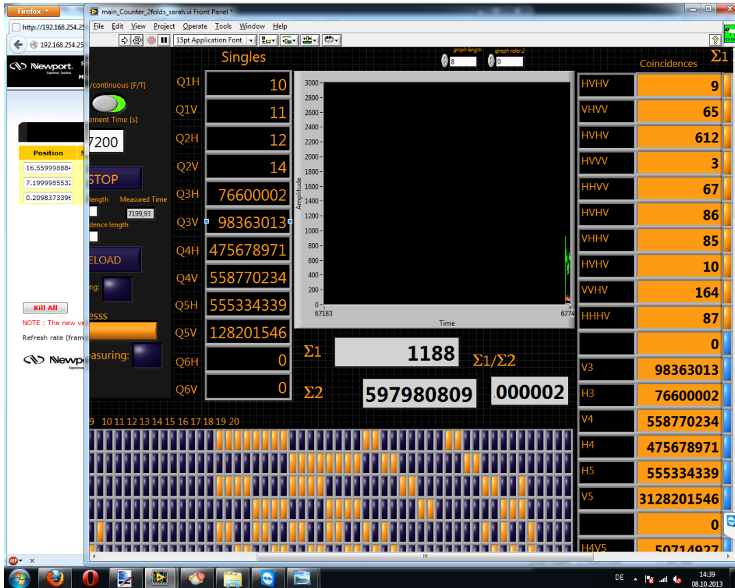
FIGURE 3.13: Screen shot of the measurement program. On the left side the 10 output combinations are recorded as coincidences, where the forth “V” stands for a count at the trigger detector. Beneath, the single counts for all five outputs (V3, H3, V4, H4, H5) and the trigger detector (V5) are measured. \Sigma 1 shows the sum of the coincidences and \Sigma 2 the sum of all single counts. On the right side, in a different window, the position of the delays can be set. This can all be done via remote control.
