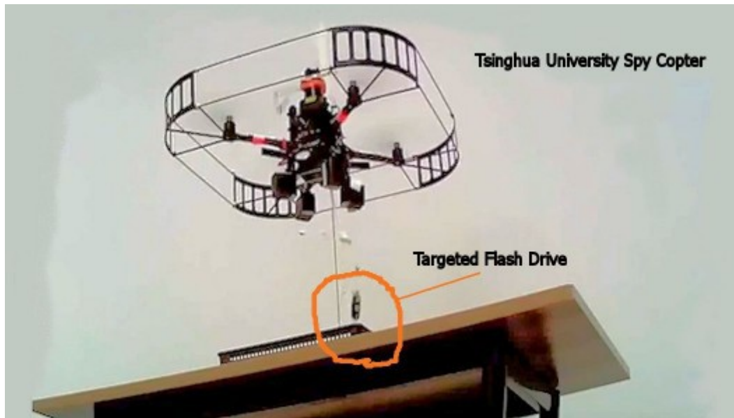
Illustration 1: Winning quadcopter design from Beijing Tsinghua University was able to navigate fully autonomous in close quarter space
