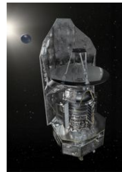
Figure 1: A computer generated view of the Herschel Space Observatory at L2, with adjusted position of shield to block off solar radiation. Picture by ESA 1
