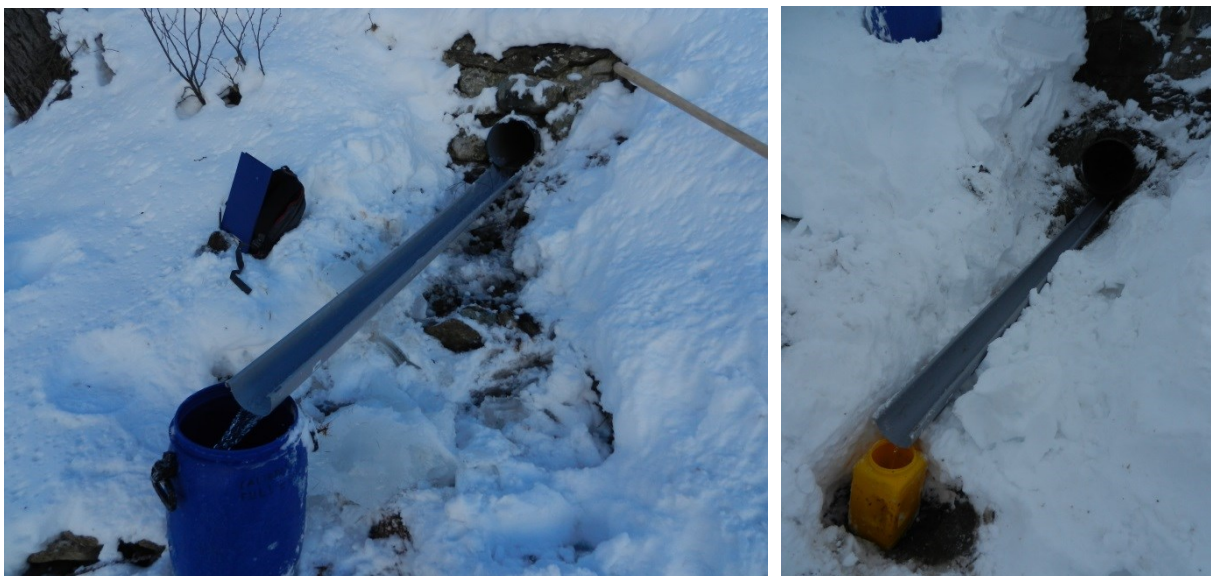
Figure 18 & Figure 19: Bucket measurements at MP D5 and MP A 21
