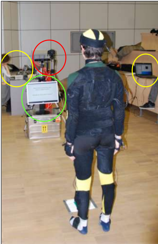
Fig.8 Experimental setup. Yellow circles – the PCs operating AnimaZoo and Kinect; green circle – video presentation display; red circle – Kinect device and a camera
