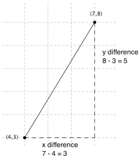
$$\text{gradient} = \frac{5}{3} = \frac{y \text{ difference}}{x \text{ difference}} \quad [ \text{Steigung} = \frac{5}{3} = \frac{y \text{ Differenz}}{x \text{ Differenz}} ]$$
