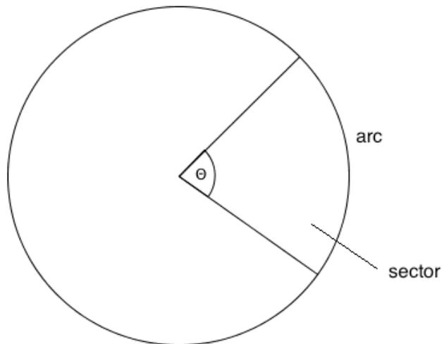
$$\text{length of arc} = \frac{\theta}{360^\circ} \times \pi D$$
