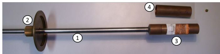
Figure 10: Photograph of the dipstick, used for measurements in the He-dewar. The metallic tube (1) contains the wires for the electrical connection. It goes through the flange (2), at which it can be fixated. The sample is mounted in the notch of the copper cylinder (3), which is then closed by the copper cup (4).
