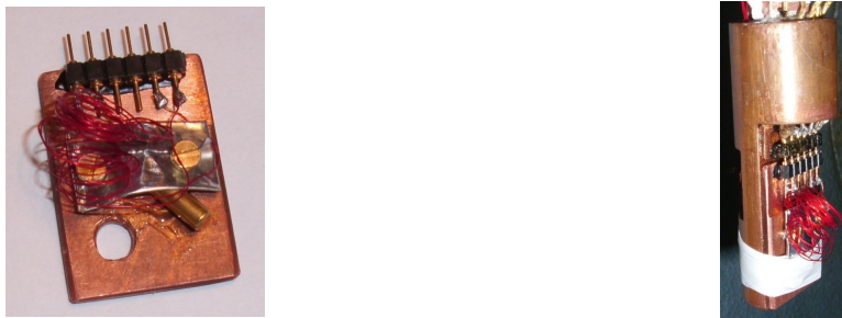
Figure 54: The calibration sensor mounted on the sample-holder (left) and in the cryostat (right).
