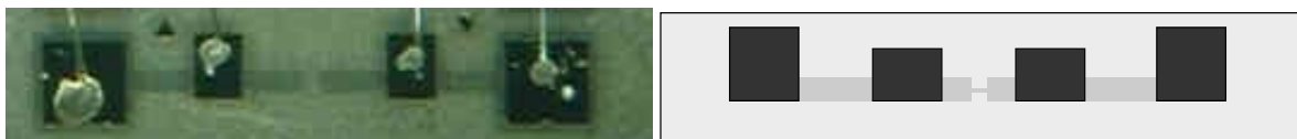
Figure 17: Photograph and scheme of one superconducting stripe of the first set of samples.
