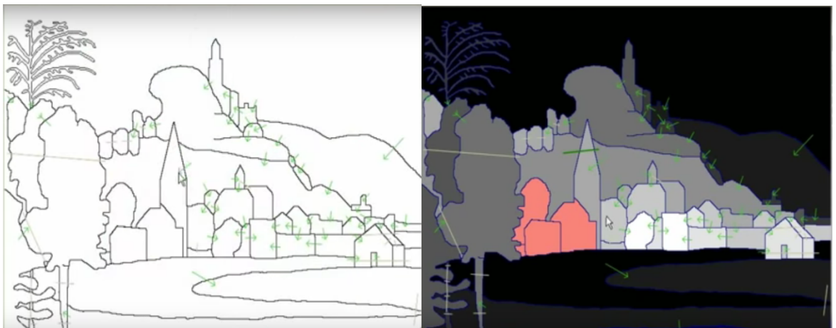
Figure 2- Height depth arrows (left) and height map with unassigned section highlighted in peach colour (right)
