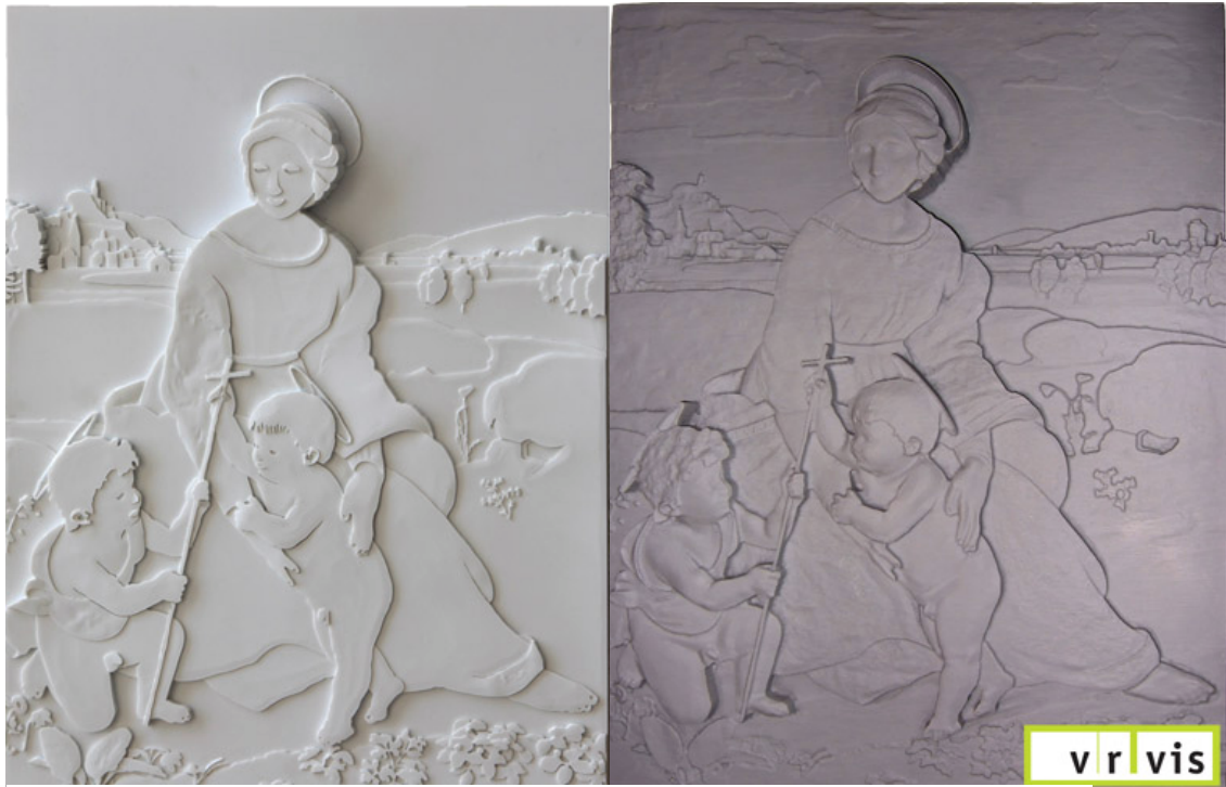
Figure 3- Layered depth diagram, a result after the first printing process (Left) and Textured Relief model, the final product of both printing processes (Right)
