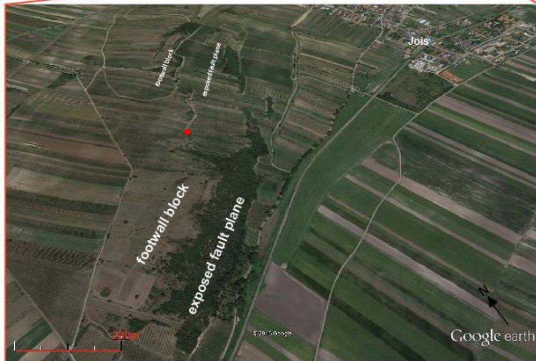
Figure 7.7. Above: geologic map of the NW part of the Neusiedlersee and the Leitha Mountains (Häusler et al., 2010) highlighting an isolated outcropping basement high just SW of the village Jois in northern Burgenland. Below: Oblique Google Earth image, looking towards the NE of the exposed footwall of en-echelon fault blocks trending NE-SW with the fault planes dipping to the SE, towards the Neusiedlersee.
