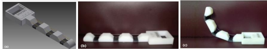
Figure 1.2: Demonstrates the possibility of printing smart material on an example official called: "Robotic Finger". We can see: a) a computer-aided design/visualization, b) a printed prototype, and c) the "finger" activated by a sliding joint https://www.researchgate.net/publication/262818283_The_Next_Wave_4D_Printing_Programming_the_Material_World
