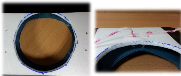
Four holes are drilled through the tray and the foil as depicted in the illustration (left). The holes in the plastic bag are supported by a piece of duct tape. Threads are threaded through the holes and are knotted on the top. A small gap is created between the underground and the plastic. This is where an air cushion can form – the reason why it is able to hover.
