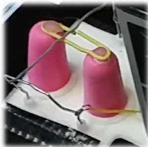
Foam ear plugs are used for the time delay switch. A bent paper clip serves for manipulating the switch in its extended state. Hot glue is used to stick the paper clip to the tips of the ear plugs. By pressing down the ear plugs, a time delay can be realized. The long piece of wire is pushed against the metal bow, by the re-expanding foam ear plug.
