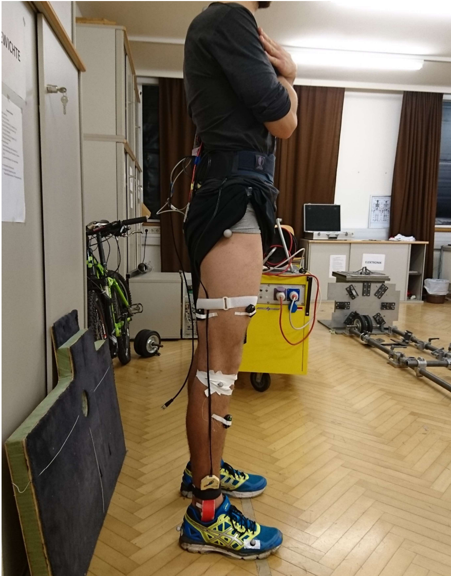
Figure 13: Subject preparation (EMG sensors, Markers, Pedar®-x system)
