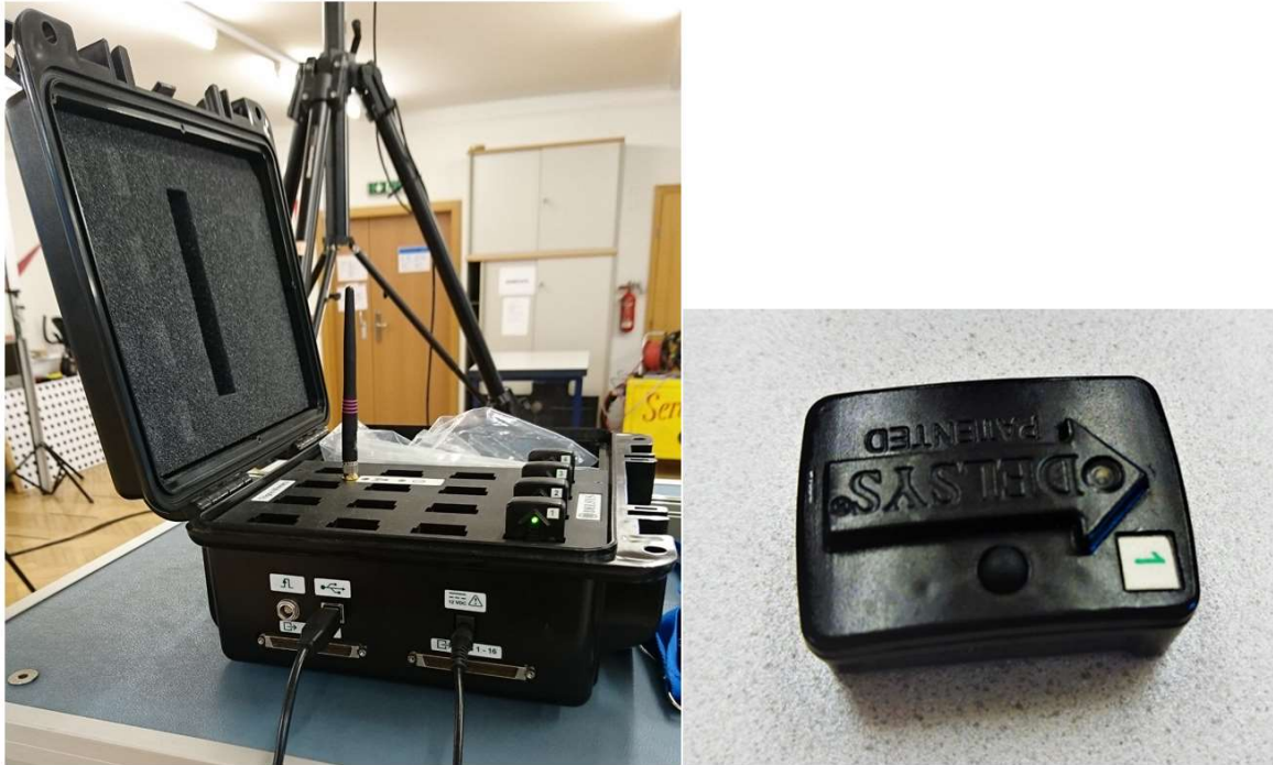
Figure 9: right: Trigno TM Wireless System from Delsys ® left: Delsys ® Sensor
